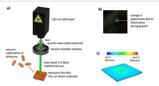
Fig. 1 (a) Schematic of the setup for tetracene growth involving laser illumination. (b) Photograph in natural light of a ca 10 mm  $\times$  10 mm tetracene sample, which was grown under laser illumination, exhibiting a spot of  $\approx 1$  mm with changed appearance, where the laser hit. (c) Heat-flow simulation of the substrate heating through the laser demonstrates a  $\approx$ 11 °C rise in substrate temperature in the illuminated spot.
