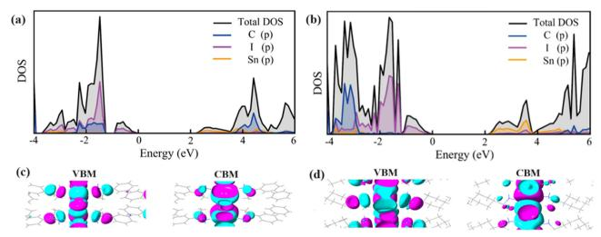
Fig. 4 Total and projected DOS of the (a) (S-MBA)<sub>2</sub>Snl<sub>4</sub> and (b) (S-CYHEA)<sub>2</sub>Snl<sub>4</sub> using the HSE06 functional. The Fermi level is designated as zero. (c) and (d) Charge densities calculated at the valence band maximum (VBM) and conduction band minimum (CBM) of both 2D layered perovskites (isovalue  $\pm 0.03$  e Å<sup>-3</sup>).
