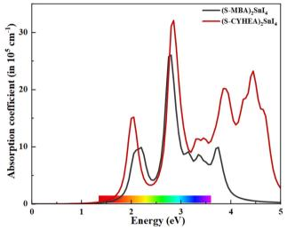
Fig. 5 Calculated absorption coefficient spectra of (S-MBA)<sub>2</sub>SnI<sub>4</sub> and (b) (S-CYHEA)<sub>2</sub>SnI<sub>4</sub> systems using the HSE06 functional without SOC.
