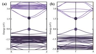
Fig. 3 Calculated band structure of (a) (S-MBA)<sub>2</sub>SnI<sub>4</sub> and (b) (S-CYHEA)<sub>2</sub> Snl₄ by GGA GGA-PBE without SOC.
