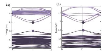
Band structure of chiral (a) (S-MBA)<sub>2</sub>SnI<sub>4</sub> (b) (S-CYHEA)<sub>2</sub>SnI<sub>4</sub> along the high symmetry directions of Brillouin zone. Light purple and black curves for CB and VB band, respectively.
