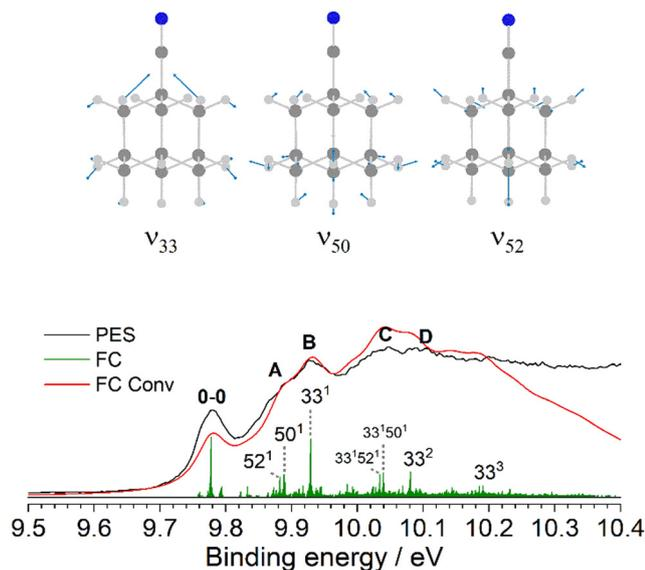
Fig. 5 The  $D_0(^2A) \leftarrow S_0(^4A_1)$  transition band from the PES spectrum of AdCN (black) compared to the simulated FC stick spectrum (green) at 340 K, which is convoluted with a FWHM of 40 meV (red). The observed vibronic features are assigned to the calculated vibrational modes  $\nu_{33} = 1221$ ,  $\nu_{50} = 890$ , and  $\nu_{52} = 848 \text{ cm}^{-1}$ .
