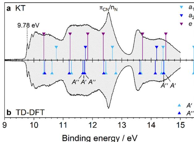
Fig. 4 PES spectrum of AdCN assigned by DFT. In panel (a), the spectrum is assigned by the KT method. In panel (b), TD-DFT is used to calculate the vertical transition energies of  $\text{AdCN}^+$  in the  $D_{0^*}$  geometry. The transition energies are shifted by the calculated first IE<sub>v</sub> (10.34 eV). The MO eigenvalues in (a) are then shifted by 0.82 eV to have the same origin as the TD-DFT method.
