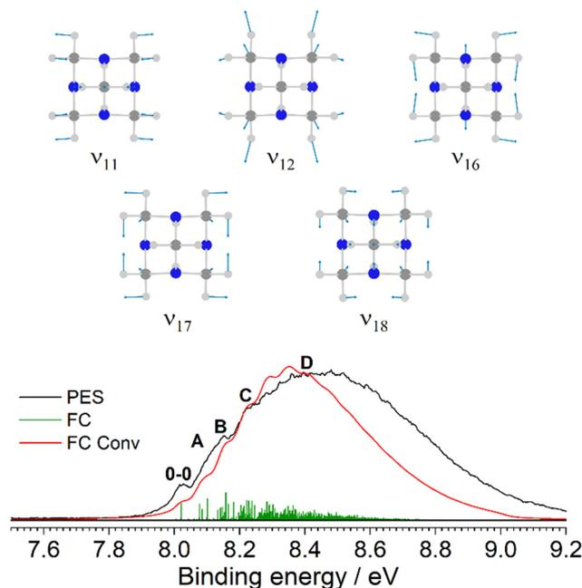
Fig. 13 The  $D_0(^1B_1) \leftarrow S_0(^2A_1)$  transition band from the PES spectrum of Uro (black) compared to the simulated FC stick spectrum (green) at 345 K, which is convoluted with a FWHM of 40 meV (red). The observed vibronic features are in close agreement with the calculated vibrational frequencies  $\nu_{11} = 1065$ ,  $\nu_{12} = 1019$ ,  $\nu_{16} = 647$ ,  $\nu_{17} = 518$ , and  $\nu_{18} = 451\text{ cm}^{-1}$ .
