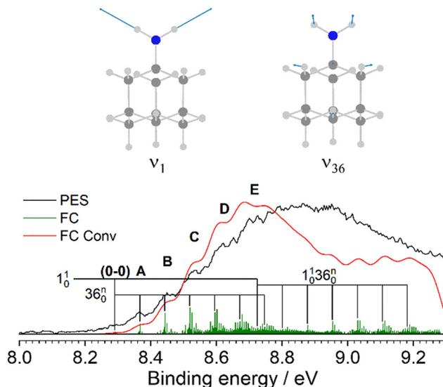
Fig. 7 The D<sub>0</sub>(<sup>2</sup>A') ← S<sub>0</sub>(<sup>1</sup>A') transition band from the PES spectrum of AdNH<sub>2</sub> (black) compared to the simulated FC stick spectrum (green) at 310 K, which is convoluted with a FWHM of 40 meV (red). The observed vibronic features are in close agreement with the calculated vibrational frequencies ν<sub>1</sub> = 3505 and ν<sub>36</sub> = 615 cm<sup>-1</sup>.
