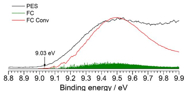
Fig. 9 The  $D_0(2A') \leftarrow S_0(1A')$  transition band from the PES spectrum of 1-AdOH (black) compared to the simulated FC stick spectrum (green) at 335 K, which is convoluted with a FWHM of 40 meV (red).
