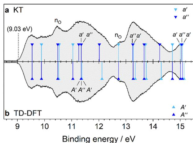
Fig. 8 PES spectrum of 1-AdOH assigned by DFT. In panel (a), the spectrum is assigned by the KT method. In panel (b), TD-DFT is used to calculate the vertical transition energies of 1-AdOH<sup>+</sup> in the  $D_0^*$  geometry. The transition energies are shifted by the calculated  $\text{IE}_v$  (9.54 eV). The MO eigenvalues in (a) are then shifted by 0.79 eV to have the same origin as the TD-DFT method.
