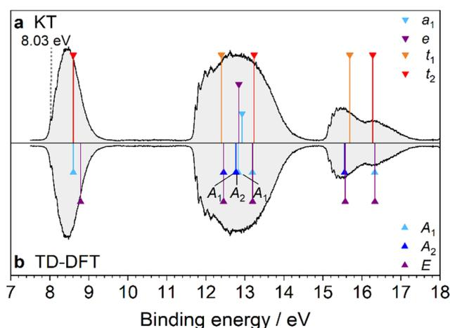
Fig. 12 PES spectrum of Uro assigned by DFT. In panel (a), the spectrum is assigned by the KT method. In panel (b), TD-DFT is used to calculate the vertical transition energies of  $Uro^+$  in the  $D_0^*$  geometry. The transition energies are shifted by the calculated  $IE_v$  (8.60 eV). The MO eigenvalues in (a) are then shifted by 0.84 eV to have the same origin as the TD-DFT method.
