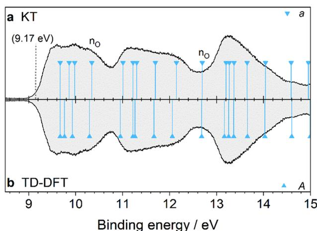
Fig. 10 PES spectrum of 2-AdOH assigned by DFT. In panel (a), the spectrum is assigned by the KT method. In panel (b), TD-DFT is used to calculate the vertical transition energies of 2-AdOH<sup>+</sup> in the  $D_0^*$  geometry. The transition energies are shifted by the calculated  $IE_v$  (9.67 eV). The MO eigenvalues in (a) are then shifted by 0.83 eV to have the same origin as the TD-DFT method.
