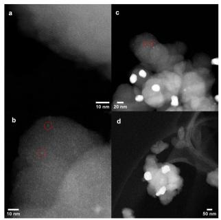
Fig. 1 HAADF-STEM micrographs of (a) Pd in (NH<sub>2</sub>)<sub>2</sub>-UiO-66, (b) and (c) Pd in CH<sub>3</sub>-UiO-66 and (d) Pd in (CH<sub>3</sub>)<sub>2</sub>-UiO-66 demonstrating the extent of embedment of Pd (bright spots) in the frameworks. Some examples of the Pd NCs have been circled, with NPs apparent as large bright areas in (c) and (d).
