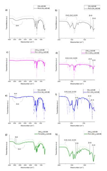
Fig. 3 FTIR spectra of Pd-laden MOFs compared with the empty parent framework: (a) and (b) CH<sub>3</sub>-UiO-66, (c) and (d) (CH<sub>3</sub>)<sub>2</sub>-UiO-66, (e) and (f)  $NH_2$ -UiO-66, and (g) and (h)  $(NH_2)_2$ -UiO-66
