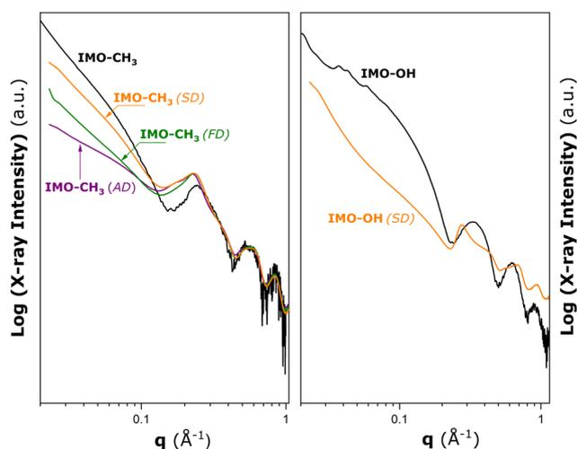
**Fig. 2** Results of SAXS measurements made on hybrid IMO-CH<sub>3</sub> (left panel) and IMO-OH (right panel) materials obtained by different drying procedures after the synthesis stage: ambient drying at 323 K (AD), freeze drying (FD), and spray drying (SD). The black solid lines represent the SAXS patterns for IMO-OH and IMO-CH<sub>3</sub> nanotubes dispersed in water added here for comparison purposes (*cf.*, Fig. S3 in the ESI†).
