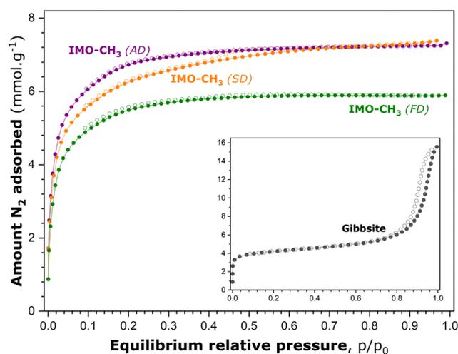
Fig. 3 Nitrogen adsorption (solid circles) and desorption (empty circles) isotherms determined for various degassed imogolite samples, before adsorption measurements, by vacuum treatment ( $10^{-5}$  mbar) at 473 K. The inset shows the corresponding curves for the gibbsite sample degassed under the same conditions.
