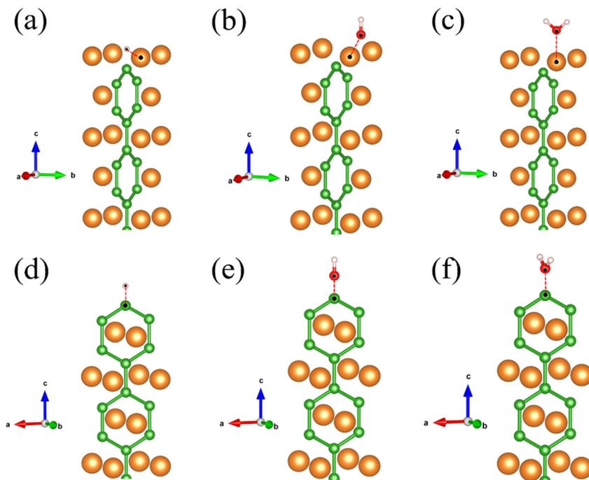
Fig. 4 (a) Mg-terminated slab adsorbing H on the hole site; (b) Mg-terminated slab adsorbing OH on the bridge site; (c) Mg-terminated slab adsorbing H<sub>2</sub>O on the top site; (d) B-terminated slab adsorbing H on the top site; (e) B-terminated slab adsorbing OH on the top site; (f) B-terminated slab adsorbing H<sub>2</sub>O on the top site. The red dashed lines represent the distance from the surface adsorbed atom to the surface atom, and the distance values are shown in Table 1.
