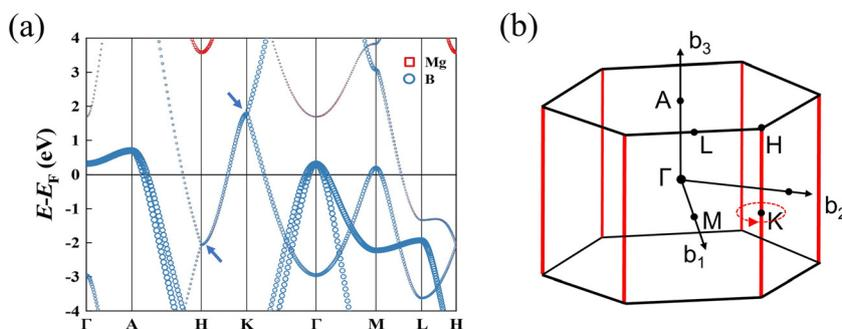
Fig. 2 (a) The calculated band structures of  $\text{MgB}_2$ , the bands are all doubly degenerate along the high-symmetric H–K path without considering the spin–orbit coupling (SOC). The degenerate bands are contributed by B atoms; (b) the nodal lines of  $\text{MgB}_2$  in the first BZ, which are along the high-symmetric H–K edges (red line). The Berry phase associated with the nodal line is  $\pi$ .
