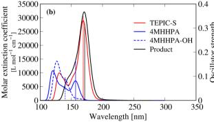
Fig. 5 Calculated ultraviolet-visible spectrum. (a) Conventional aromatic epoxy (DGEBA) and three types of TEPIC resins. (b) Reactants and product.
