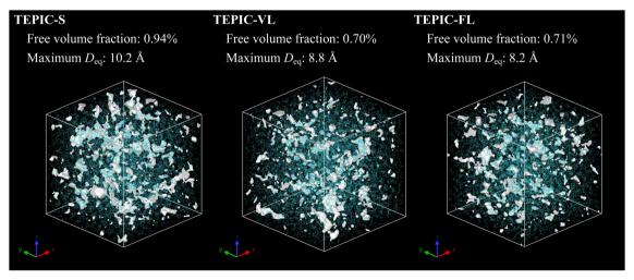
Fig. 10 Snapshots of free volume distributions of three resin types at the same strain level in triaxial tensile simulations.
