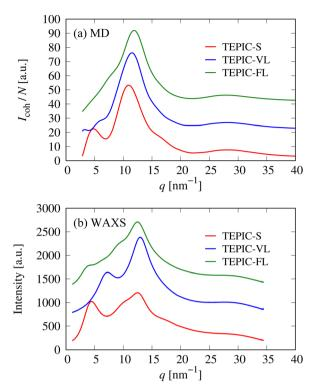
Fig. 11 Comparison of X-ray scattering intensities of three types of resins obtained from (a) MD simulations and (b) WAXS.
