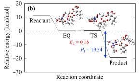
Fig. 7 Reaction pathways and reaction energies of the (a) first and (b) second reactions
