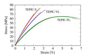
Fig. 8 Stress-strain curves in the unitensile experiment.
