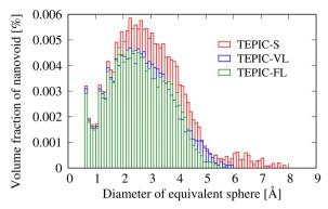
Fig. 12 Size distributions of the free volumes of three types of resins in terms of the diameters of the volume-equivalent spheres.
