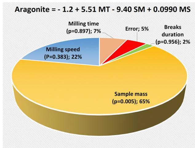
Fig. 2 Analysis of variance (ANOVA) results showing the contributions of individual milling parameters (in %) to the degree of phase transformation in eggshell (aragonite content) and  $p$  values. The regression is also included: MT – milling time, h; MS – milling speed, rpm; SM – sample mass, g.
