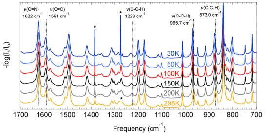
Fig. 2 FTIR spectra at varying temperatures for COF-300. Peaks marked with an asterisk are from H<sub>2</sub>O and CO<sub>2</sub> contaminants in the KBr pellets and not from the samples under investigation. Spectra from 4000-700 cm<sup>-1</sup> are given in Fig. S22 (ESI†).
