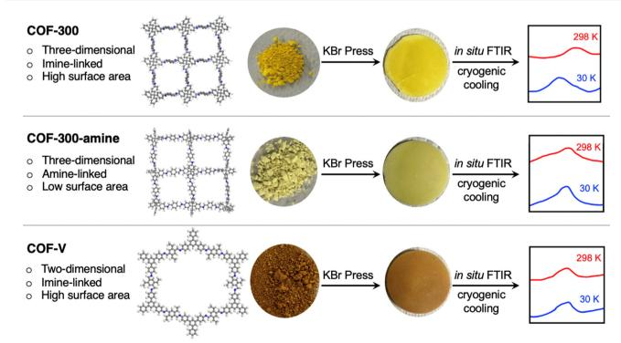
Fig. 1 Schematic depiction of the in situ FTIR analysis performed on three covalent organic frameworks. The image of the COF-300 structure was created from crystallographic data published in ref. 28; the images of the COF-300-amine and COF-V structures are simply illustrations created using the program Materials Studio.
