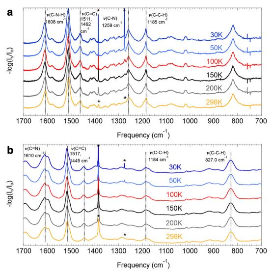
Fig. 5 FTIR spectra at varying temperatures for COF-300-amine (a) and COF-V (b). Peaks marked with an asterisk are from H<sub>2</sub>O and CO<sub>2</sub> contaminants in the pellets and not from the samples under investigation. Spectra from 4000-700 cm<sup>-1</sup> are given in Fig. S23 and S24 (ESI†).
