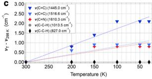
**Fig. 4** Peak shifts as a function of temperature for COF-300 (a), COF-300-amine (b), and COF-V (c). Symbols are the peak shift for each temperature T and dotted lines are the linear fit for the temperature dependence of the shift for each mode, which was constrained to intersect 0 cm $^{-1}$  at room temperature.
