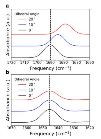
Fig. 7 Simulated IR peaks for varying dihedral angles in N-benzylideneaniline (a) and N-benzylaniline (b). Shown are just a portion of the spectrum; the C=N stretch in (a) and the C-N-H bend in (b).
