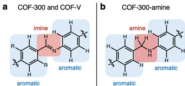
Fig. 3 Depiction of the functional groups containing the vibrational modes analyzed herein for COF-300 (a; R = H), COF-V (a; R = CHCH<sub>2</sub>), and COF-300-amine (b).
