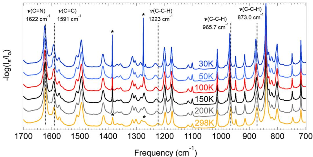
Fig. 2 FTIR spectra at varying temperatures for COF-300. Peaks marked with an asterisk are from H<sub>2</sub>O and CO<sub>2</sub> contaminants in the KBr pellets and not from the samples under investigation. Spectra from 4000–700 cm<sup>-1</sup> are given in Fig. S22 (ESI<sup>†</sup>).
