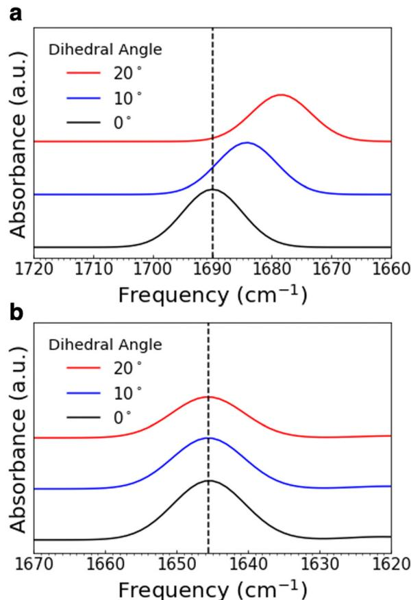
**Fig. 7** Simulated IR peaks for varying dihedral angles in *N*-benzylideneaniline (a) and *N*-benzylaniline (b). Shown are just a portion of the spectrum; the C=N stretch in (a) and the C-N-H bend in (b).
