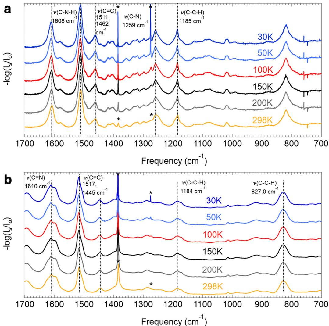
Fig. 5 FTIR spectra at varying temperatures for COF-300-amine (a) and COF-V (b). Peaks marked with an asterisk are from H<sub>2</sub>O and CO<sub>2</sub> contaminants in the pellets and not from the samples under investigation. Spectra from 4000–700 cm<sup>-1</sup> are given in Fig. S23 and S24 (ESI<sup>†</sup>).
