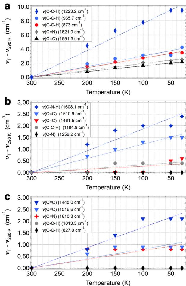
Fig. 4 Peak shifts as a function of temperature for COF-300 (a), COF-300-amine (b), and COF-V (c). Symbols are the peak shift for each temperature  $T$  and dotted lines are the linear fit for the temperature dependence of the shift for each mode, which was constrained to intersect  $0 \text{ cm}^{-1}$  at room temperature.
