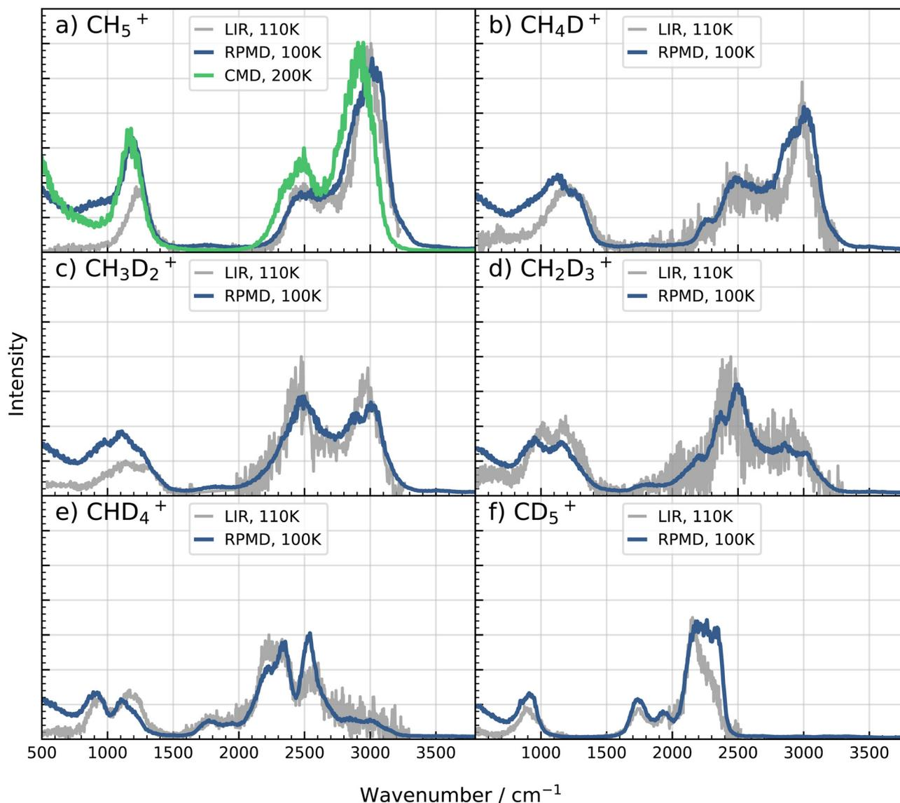
Fig. 1 Infrared spectra of  $\text{CH}_5^+$  and its deuterated isotopologues up to  $\text{CD}_5^+$  computed from RPMD (blue) and CMD (green) path integral simulations at CCSD(T) accuracy, see text. The corresponding experimental reference spectra (gray) were obtained from laser induced reactions (LIR) action vibrational spectroscopy as published in ref. 14 the arbitrary intensity scale of the LIR spectra has been adjusted individually to allow for easy comparison to the computed IR spectra.
