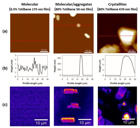
Fig. 3 (a) AFM representative 30  $\mu$ m  $\times$  30  $\mu$ m topography images of Tstilbene-containing PS films. (b) Intensity profiles (the distance in the Z direction from the film surface) along the red lines indicated in (a). (c) CARS images of the same films at 1600 cm $^{-1}$  in the similarly sized 30  $\mu$ m  $\times$  30  $\mu$ m range.
