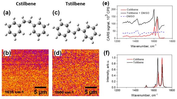
Fig. 1 Chemical structures of Cstilbene (a) and Tstilbene (c). CARS images, captured at a resonance frequency of 1635 cm<sup>-1</sup> for pure Cstilbene, (b) and diluted solution of Tstilbene in DMSO (d) with a resonance frequency of 1600 cm<sup>-1</sup>. Measured CARS spectra of pure Cstilbene and mono-molecular Tstilbene (e). CARS spectrum of DMSO is shown for reference. Calculated Raman spectra of Cstilbene and Tstilbene molecules (f)
