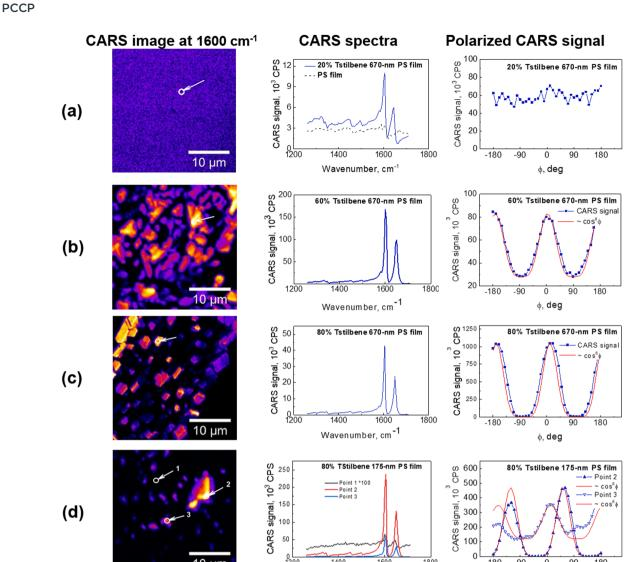
Fig. 2 Left: CARS images of various films of Tstilbene and PS mixtures at 1600 cm<sup>-1</sup>. Middle: CARS spectra at the selected points indicated with arrows. Right: Polarized CARS signal measured at  $1600 \text{ cm}^{-1}$  at the same selected spatial point. Each data point is the result of averaging over an area of about  $1 \mu m^2$  at the chosen position of the sample (a)-(d). The types of films are indicated in the middle panels.
