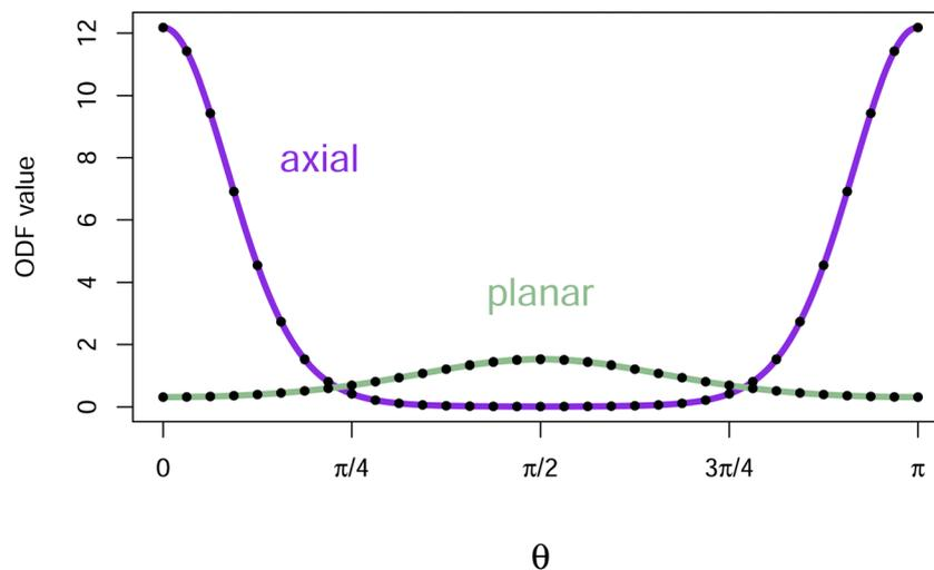
Fig. 6 Planar and axial ODFs from the iterative method for the Maier–Saupe kernel with  $B = 9$ , compared with exact values from the analytical solutions<sup>20</sup> plotted as black dots. The Maier–Saupe kernel gives results qualitatively similar to the Onsager kernel ( $W(\gamma) = \sin(\gamma)$ ) while being more amenable to analysis, and this is reflected in the similarity between Fig. 2 and 6.
