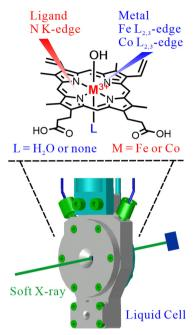
Fig. 1 A schematic of the liquid cell for XAS of metalloporphyrins in aqueous solutions. XAS spectra of central metals in metalloporphyrins were obtained at the Fe or Co L<sub>2,3</sub>-edge and those of ligands were obtained at the N K-edge, respectively. The hydration of the metalloporphyrin was also investigated by the N K-edge XAS.
