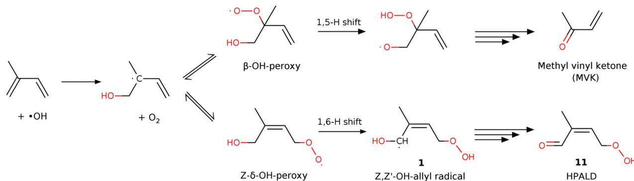
Fig. 1 A simplified reaction schematic of the reaction pathways in the LIM1 model after the addition of O<sub>2</sub> to the isoprene-OH radical for case I.
