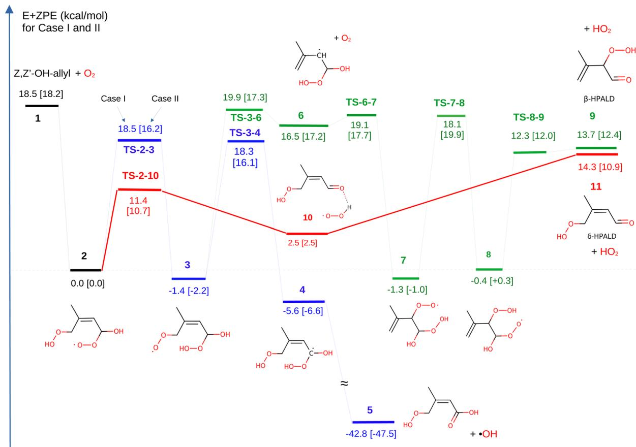
Fig. 3 Potential energy profiles for the  $Z,Z'$ -allyl radical +  $O_2$  reactions. Zero-point corrected energies are given in kcal mol<sup>-1</sup> for case I and in brackets for case II. The structures of the intermediates and products are displayed only for case II.
