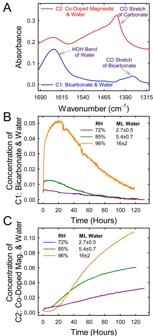
Fig. 2 Results from a two-component MCR-ALS analysis of the combined spectra from TDep\_1 at 96% RH, TDep\_2 at 85% RH, and TDep\_3 at 72% RH. Components C1 and C2 are shown in (A) and are assigned to bicarbonate and Co-doped magnesite, respectively. Water is also present in both components. The concentrations of C1 and C2 are shown in (B) and (C), respectively, for each experiment.
