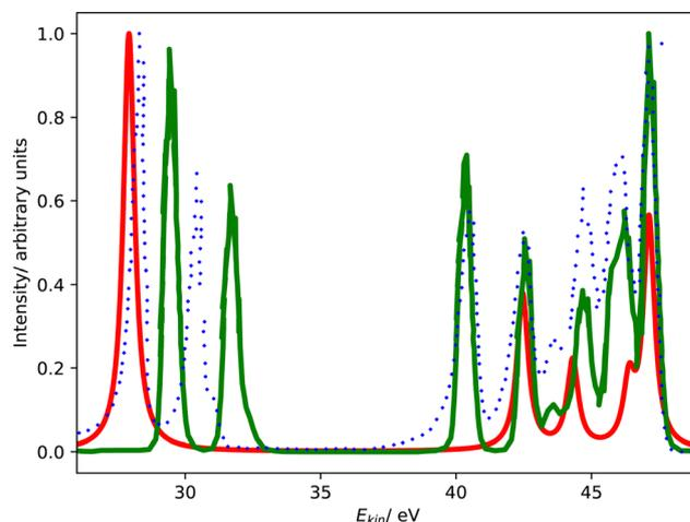
Fig. 2  $L_1L_{2,3}M$  Coster–Kronig spectrum of argon. Comparison of CS-EOM-CCSD results (red solid line, this work) with MCDHF results (green solid line, ref. 25) and the experimental spectrum (blue dotted line, ref. 25). The theoretical spectra are shifted to higher kinetic energy by 3.4 eV and 1.3 eV, respectively.
