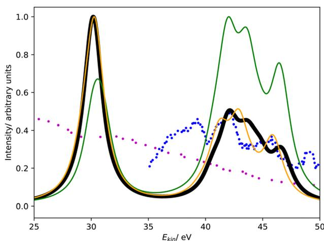
Fig. 3  $L_{1,2,3}M$  Coster-Kronig spectrum of hydrogen sulfide. Partial decay widths were computed with CBF-EOM-CCSD (black solid line), Fano-EOM-CCSD (orange solid line), and assuming the same width for every channel (green solid line). The experimental data reported in ref. 47 and 46 are shown as blue and purple dotted lines. The theoretical spectra are shifted to higher kinetic energy by 7.5 eV.
