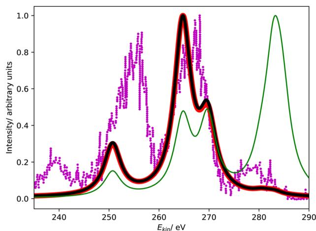
Fig. 4  $L_1MM$  Auger spectrum of argon. Partial decay widths were computed with CS-EOM-CCSD (red solid line), CBF-EOM-CCSD (black solid line), and assuming the same width for every channel (green solid line). The experimental spectrum reported in ref. 25 is shown as purple dotted line. The theoretical spectra are shifted to higher kinetic energy by 2.0 eV.
