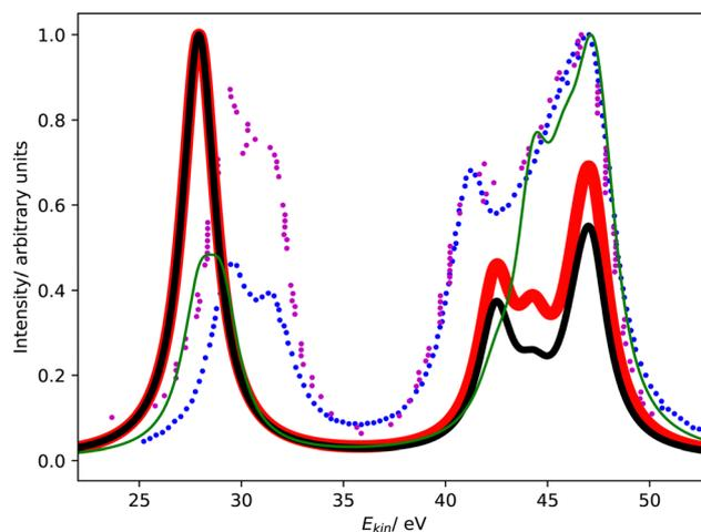
Fig. 1  $L_1L_{2,3}M$  Coster–Kronig spectrum of argon. Partial decay widths were computed with CS-EOM-CCSD (red solid line) and CBF-EOM-CCSD (black solid line), and assuming the same width for every channel (green solid line). The experimental Coster–Kronig spectra reported in ref. 23 and 25 are shown as blue and purple dotted lines, respectively. The theoretical spectra are shifted to higher kinetic energy by 3.4 eV.
