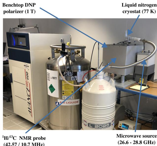
**Fig. 8** A visual representation of the entire benchtop DNP polarizer setup. The location of the main hardware components (the magnet, the cryostat, the microwave source, the DNP-NMR probe) are highlighted using arrows.
