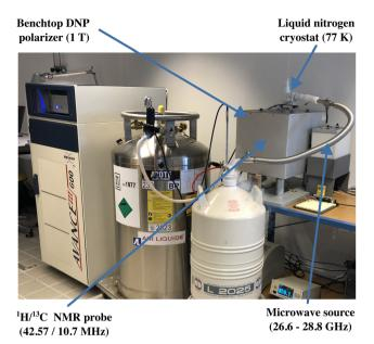
Fig. 8 A visual representation of the entire benchtop DNP polarizer setup. The location of the main hardware components (the magnet, the cryostat, the microwave source, the DNP-NMR probe) are highlighted using arrows.
