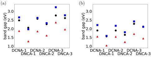
Fig. 3 Band gaps of (a) DA-COFs and (b) protonated DA-COFs obtained from experiment<sup>20</sup> (black circles) and calculated using PBE (red triangles) and HSE (blue squares).
