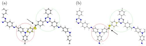
Fig. 8 Spin densities (yellow) after hydrogen adsorption at (a) DCNA-1 and (b) DNCA-1. An isosurface level of 0.01 eV Å<sup>-3</sup> was used. The arrow indicates the adsorbed hydrogen. Donor and acceptor groups as defined for the charge analysis in Table 2 are indicated in red and green, respectively,
