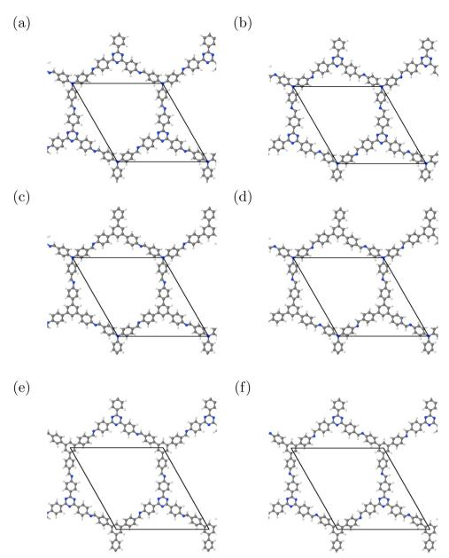
Fig. 1 Structures of (a) DCNA-1, (b) DNCA-1, (c) DCNA-2, (d) DNCA-2, (e) DCNA-3, (f) DNCA-3, optimized at the PBE+D3 level of theory. H: white; C: grey; N: blue. Solid lines indicate hexagonal elementary cells used in simulations. The optimized values for a (=b) are 23.22, 23.26, 23.43, 23.48, 25.47, and 25.50 Å for DCNA-1, DNCA-1, DCNA-2, DNCA-2, DCNA-3, and DNCA-3, respectively. The angle  $\gamma$  is 119.6° for DCNA-3 and DNCA-3 and 120.0° for the other COFs.
