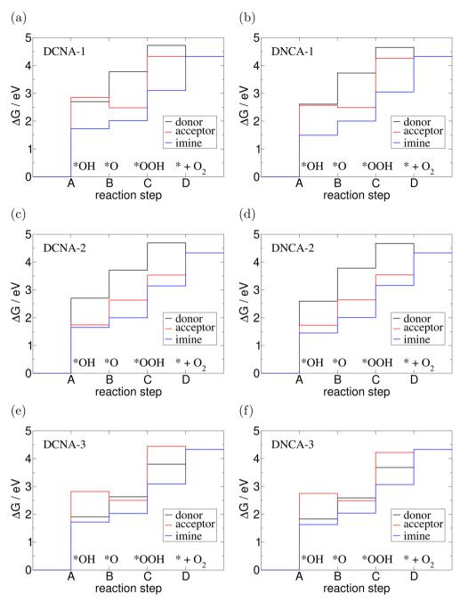
OER reaction profiles of (a) DCNA-1, (b) DNCA-1, (c) DCNA-2, (d) DNCA-2, (e) DCNA-3, (f) DNCA-3
