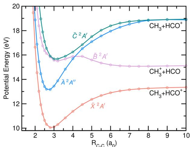
**Fig. 8** Potential energy curves of cationic acetaldehyde as a function of the C–C bond distance (in atomic units,  $a_0$ ) for the first four electronic states,  $\tilde{X}^2A'$ ,  $\tilde{A}^2A''$ ,  $\tilde{B}^2A'$  and  $\tilde{C}^2A'$ . The two first dissociation limits correspond to the formation of the two fragments in their respective ground electronic states while the third corresponds to the formation of  $\text{HCO}^+$  in its first excited electronic state.
