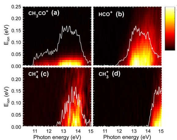
**Fig. 5** Ion signal correlated to threshold photoelectrons as a function of ion kinetic energy,  $E_{\text{ion}}$  and photon energy for (a)  $\text{CH}_3\text{CO}^+$ , (b)  $\text{HCO}^+$ , (c)  $\text{CH}_4^+$ , and (d)  $\text{CH}_3^+$ . The photon energy axis corresponds to the ionization energy since only threshold electrons are considered. The TPES obtained for  $E_{\text{ion}}$  below 25 meV is plotted as white curves. The color bar on the right represents the intensity (in arb. units).
