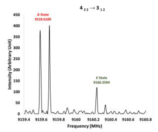
Fig. 3 The  $4_{22} \rightarrow 3_{12}$  transition of PhAc···CH<sub>3</sub>OH complex (recorded using PN-FTMW spectrometer) showing *A* and *E*-states. The transitions are further split due to the Doppler effect.
