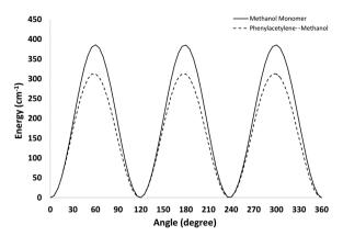
Fig. 4 The potential energy curve for the internal rotation of the  $CH_3$  group in the  $CH_3OH$  monomer (solid line) and  $PhAc\cdots CH_3OH$  complex (dashed line).
