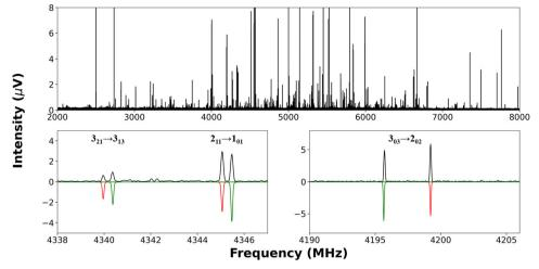
Fig. 2 (Top panel) The broadband rotational spectrum of PhAc···CH<sub>3</sub>OH complex recorded in 2.0-8.0 GHz region using CP-FTMW spectrometer. (Bottom panels) Experimentally observed transitions of the PhAc···CH<sub>3</sub>OH complex are shown (black) above the simulated spectrum (red and green colour for A- and E-states, respectively)
