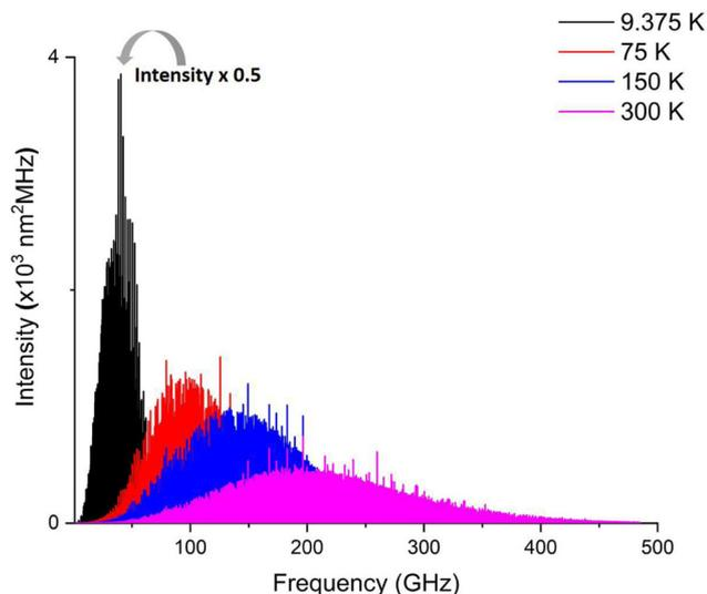
Fig. 6 Distribution of rotational transitions of CHT-1-CN-1 for four of the standard temperatures implemented in the JPL database.<sup>29</sup> The frequency simulation is made up to 500 GHz for the case of  $2I + 1 = 1$ . Note that the intensity scale for the prediction at 9.375 K has been halved for clearer comparison with the predictions at higher temperatures.
