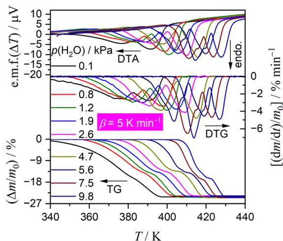
Fig. 1 TG–DTG–DTA curves depicting the thermal dehydration of CC-DH ( $m_0 = 3.02 \pm 0.04$  mg) to form CC-AH recorded at a  $\beta$  of 5  $\text{K min}^{-1}$  in a stream of wet  $\text{N}_2$  ( $q_v = 200 \text{ cm}^3 \text{min}^{-1}$ ) with different  $p(\text{H}_2\text{O})$  values ( $0.1 \leq p(\text{H}_2\text{O})/\text{kPa} \leq 9.8$ ).
