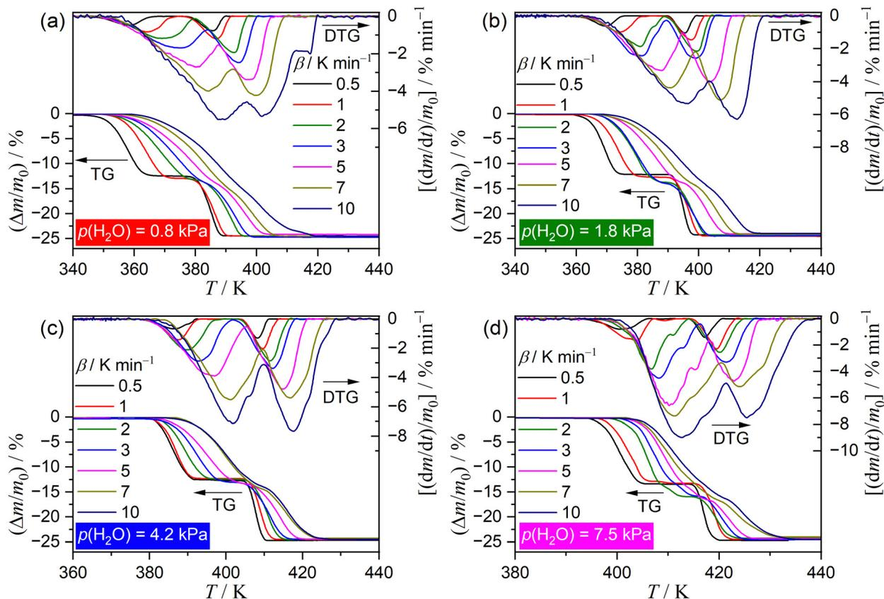
Fig. 2 TG–DTG curves depicting the thermal dehydration process of CC-DH to form CC-AH recorded at different  $\beta$  values in a stream of wet  $N_2$  with selected  $p(H_2O)$  values: (a) 0.8 kPa ( $m_0 = 3.01 \pm 0.04$  mg), (b) 1.8 kPa ( $m_0 = 3.02 \pm 0.06$  mg), (c) 4.2 kPa ( $m_0 = 3.03 \pm 0.05$  mg), and (d) 7.5 kPa ( $m_0 = 3.02 \pm 0.04$  mg).
