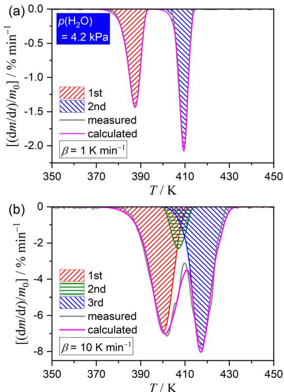
Fig. 3 Typical MDA results highlighting the two and three mass loss steps of the thermal dehydration process of CC-DH at  $p(\text{H}_2\text{O}) = 4.2$  kPa at different  $\beta$  values: (a)  $1 \text{ K min}^{-1}$  and (b)  $10 \text{ K min}^{-1}$ .
