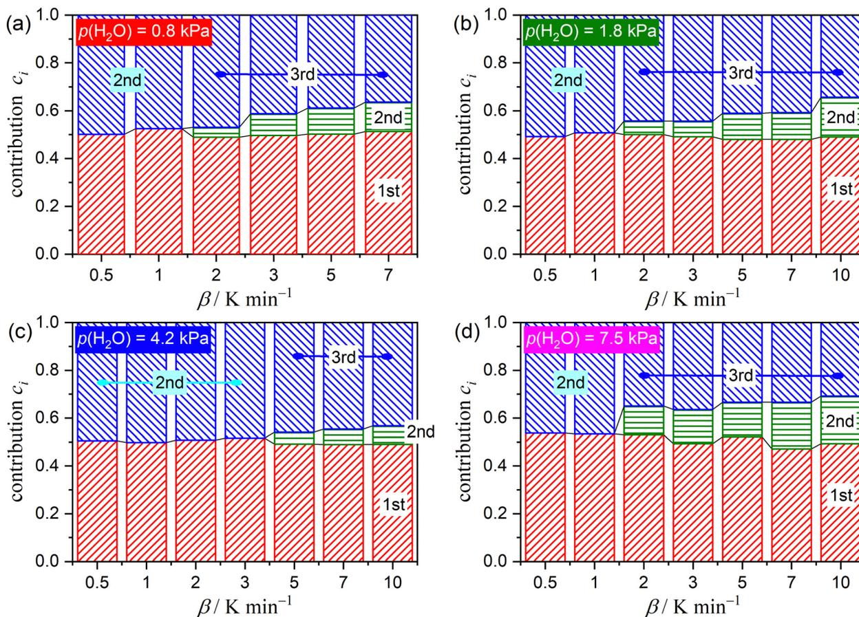
Fig. 4 Variation in contribution  $c_i$  of the component mass loss steps with  $\beta$  observed for the thermal dehydration of CC-DH to form CC-AH at individual  $p(\text{H}_2\text{O})$  values: (a) 0.8, (b) 1.8, (c) 4.2, and (d) 7.5 kPa.
