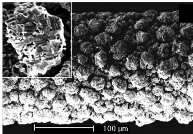
Fig. 1 Platinum catalyst surface reconstruction during ammonia oxidation. Image taken from Hannevold *et al.*<sup>8</sup>
