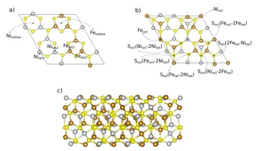
Fig. 1 Pristing pentlandite (Pn) 2 × 1 surface (111) supercell based on the energetically most favorable Pn bulk structure. All possible metal and sulfur adsorption sites are marked in panels (a) and (b). A sideview of the slab is shown in panel (c). Sulfur sites are named based on their neighboring metal atoms. Explanation of abbreviations in indices: oct is octahedral, tet is tetrahedral, and numbers as indices are used to distinguish between different sites.
