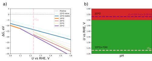
Fig. 3 (a) Stability diagram for various oxygenated phases of a non-reconstructed Pn(111) model electrode; (b) Pourbaix diagram for the Pn(111) surface where, besides the oxygenated phases, also mixed \*O/\*OH coverages are taken into account in the potential window of the oxygen evolution reaction (OER). Energetically favorable phases are 20\*O (red) and 19\*O + \*OH (green)
