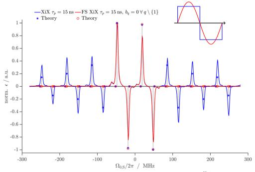
Fig. 4 DNP profile for XiX (blue line) and FS-XiX (red line) recorded at X-band (0.35 T) with a Rabi frequency of  $\frac{\omega_{1,S}}{2} = 4$  MHz and a pulse length  $\tau_p = 15$  ns (further experimental parameters are given in Section 5). The dots and asterisks represent the estimated enhancement  $\varepsilon_{\rm ZQ/DQ}$  as given in eqn (13).
