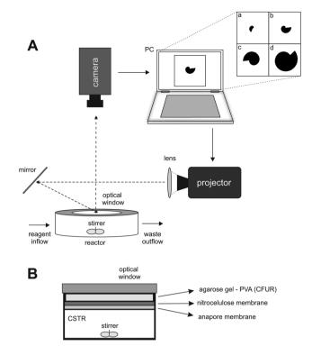
Fig. 1 (A) Schematic representation of the experimental setup. (B) Lateral view of the CSTR/CFUR reactor
