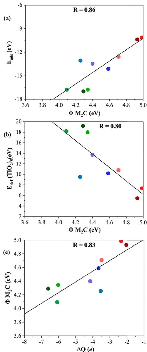
Fig. 7 (a)  $E_{ads}$  vs. the work function,  $\Phi$ , of bare (0001) MXene surfaces; (b)  $E_{def}(TiO_2)_5$  vs.  $\Phi M_2C$ ; and (c)  $\Phi M_2C$  vs.  $\Delta Q$  of  $(TiO_2)_5$ . The solid black lines correspond to the linear fitting associated with the regression coefficient,  $R$ . Color coding as in Fig. 3. Linear fitting analysis is reported in Table S12 of the ESI.†
