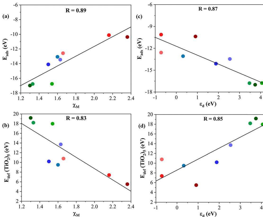
Fig. 8 Tentative linear correlations of (a)  $E_{\text{ads}}$  vs.  $\chi_{\text{M}}$ , (b)  $E_{\text{def}}(\text{TiO}_2)_5$  vs.  $\chi_{\text{M}}$ , (c)  $E_{\text{ads}}$  vs.  $\epsilon_{\text{d}}$ , and (d)  $E_{\text{def}}(\text{TiO}_2)_5$  vs.  $\epsilon_{\text{d}}$ . The linear regression coefficient,  $R$ , is given in the inset in each panel. Color coding as in Fig. 3. Linear fitting analysis is reported in Table S12 of the ESI.†
