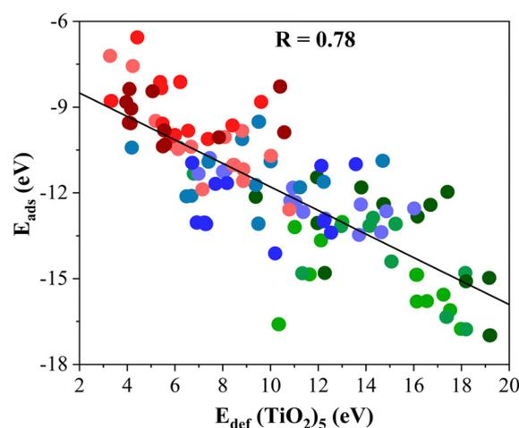
**Fig. 2** Linear trend between the  $E_{\text{ads}}$  of  $(\text{TiO}_2)_5/\text{M}_2\text{C}$  composites and  $E_{\text{def}}$  ( $\text{TiO}_2)_5$ . The solid black line is the linear correlation between both quantities where  $R$  stands for the regression coefficient between them. The spheres colors are consistent with the colored spheres of the metal atom in the MXene surface, depicted in Fig. 3. Linear fitting analysis is reported in Table S12 of the ESI.†
