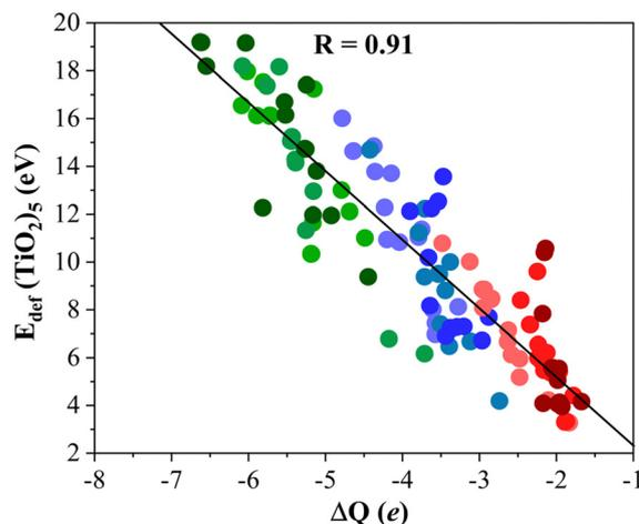
Fig. 5 Linear correlation between  $E_{\text{def}}(\text{TiO}_2)_5$  and  $\Delta Q$ . Solid black line is the linear correlation between both quantities, while  $R$  stands for the linear correlation regression coefficient. Color coding as in Fig. 3. Linear fitting analysis is reported in Table S12 of the ESI.†
