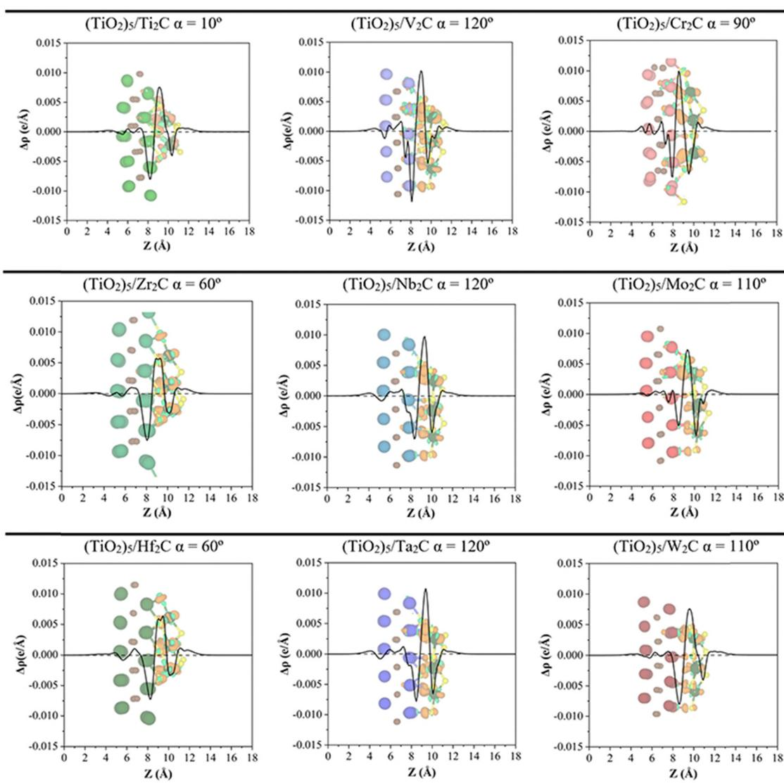
Fig. 6 Plane-averaged charge density difference (PA-CDD)  $\Delta\rho$  along the direction normal to the MXene surface,  $Z$ , for the most stable configurations of  $M_2C/(TiO_2)_5$  as listed in Table 1. Charge density differences, CDD, with an isosurface value of  $0.015 \text{ e } \text{\AA}^{-3}$ , are depicted inset where pale green and orange isosurfaces correspond to accumulation and depletion charges, respectively. Color coding as in Fig. 3.
