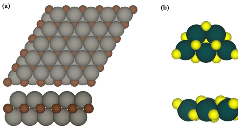
**Fig. 1** Top (top) and side (bottom) views of (a) the  $p(5 \times 5)$  supercell model of the (0001)  $\text{M}_2\text{C}$  MXene structure with an ABC stacking and (b) planar  $(\text{TiO}_2)_5$  cluster. Gray and brown spheres represent transition metal M ( $M = \text{Ti, Zr, Hf, V, Nb, Ta, Cr, Mo, and W}$ ) and C atoms in the  $\text{M}_2\text{C}$  (0001) MXene surface, while yellow and dark green spheres stand for oxygen and titanium atoms of the titania cluster, respectively.
