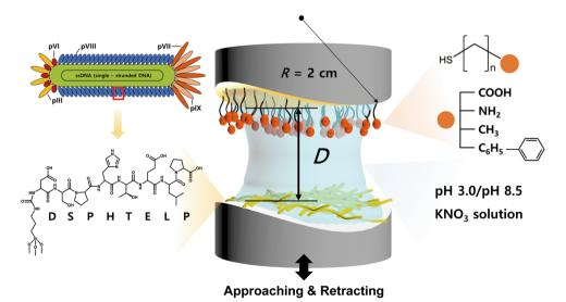
Fig. 2 Schematic of surface forces apparatus (SFA) for measuring the interaction forces between the 8-mer peptide layer (bottom surface) and four different alkanethiols' SAM layers (top surface) under various conditions.
