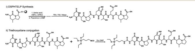
Fig. 1 Schematic representation of the synthesis of 8-mer peptides. 8-Mer peptides were synthesized by solid-phase peptide synthesis at a 0.106 mmol scale. The N-terminal of the synthesized amino acid backbones was conjugated with triethoxysilane in anhydrous DMF solvent.
