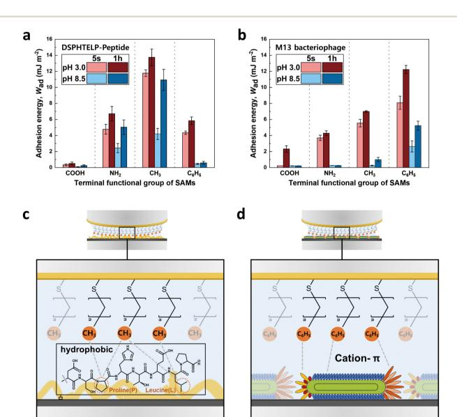
Fig. 5 Bar graph showing the adhesion energy on the (a) 8-mer peptide and (b) M13 bacteriophage layers with four different SAMs,<sup>33</sup> depending on contact time and pH; average  $\pm$  standard error bars (n = 3 in each group). Schematic representations of the interactions between (c) CH<sub>3</sub>-SAM and the 8-mer peptide and (d) C<sub>6</sub>H<sub>5</sub>-SAM and the M13 bacteriophage.
