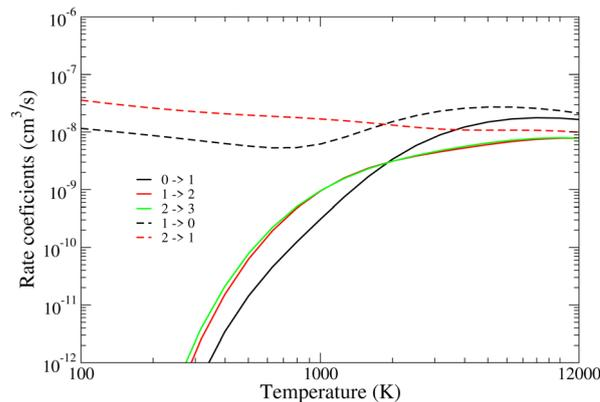
Fig. 10 VE (continuous lines) and VdE (dashed lines) cross sections of BeH<sup>+</sup> ( $\nu_i = 0-2$ ) calculated using eqn (24) from the cross sections shown in Fig. 5.
