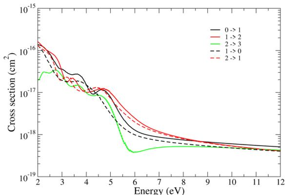
Fig. 5 VE (continuous lines) and VdE (dashed lines) cross sections for  $\text{BeH}^+$  ( $v_i = 0-2$ ) for  $\Delta v = v_f - v_i = \pm 1$  transitions.
