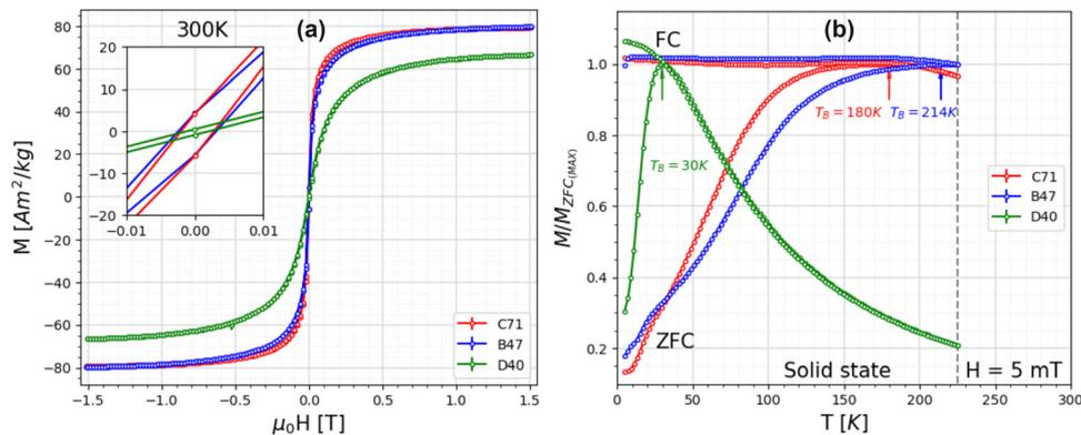
Fig. 5 (a) Hysteresis curves at room temperature in the range of  $\pm 1.5$  T. (b) Normalized ZFC/FC curves performed in the temperature range of 5–225 K and a magnetic field of 5 mT. The upper limit temperature is set at 225 K to avoid traversing the melting temperature of water.
