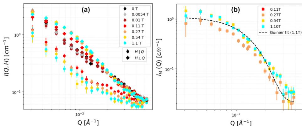
Fig. 8 (a) Scattering intensity of sample C71 dispersion in  $D_2O$  solvent in the parallel sector ( $H \parallel Q$ ) and perpendicular sector ( $H \perp Q$ ), (b) pure magnetic scattering at high fields close to saturation.
