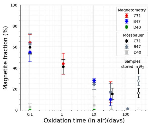
**Fig. 4** Comparison of the magnetite fraction obtained over various oxidation times in air from Mössbauer spectroscopy and magnetometry. The samples stored under N<sub>2</sub> (empty symbols) are included for comparing the magnetite fraction to the samples stored in the air.
