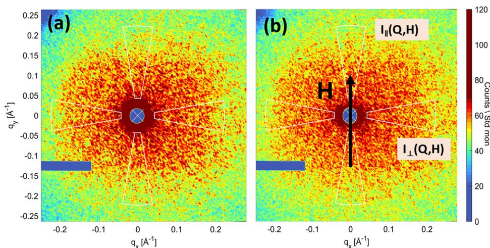
Fig. 7 Two-dimensional SANS patterns for sample C71 dispersed in  $D_2O$ . (a) Isotropic pattern with no applied magnetic field, (b) anisotropic pattern with the magnetic field of 1.1 T along the vertical direction, as shown by an arrow.
