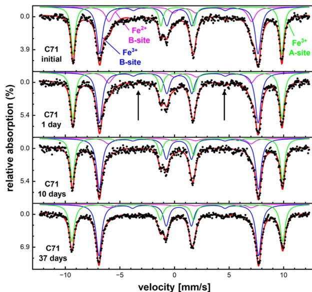
**Fig. 3** Mössbauer spectra for sample C71 after various aging times of exposure to air, recorded at 5 K and an applied magnetic field of 8 T. In the C71 1 day spectrum, the vertical arrows mark Mössbauer lines 2 and 5, whose relative intensity indicates the degree of spin canting.<sup>51</sup>
