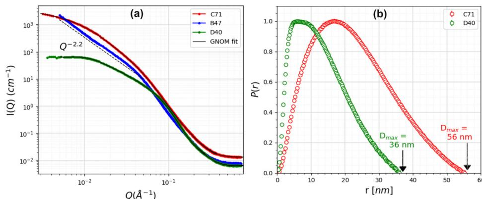
**Fig. 2** (a) SAXS curves for the diluted samples with a concentration of  $5.5 \text{ mg ml}^{-1}$  iron for the C71 and B47 samples and up to  $3.3 \text{ mg ml}^{-1}$  iron for the D40 sample, and (b) pair-distance distribution functions  $P(r)$  for samples C71 and D40, indicating that large particles are formed by the single-core nanoparticles.
