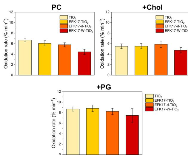
Fig. 2 C<sub>11</sub>-BODIPY oxidation rates for bare TiO<sub>2</sub> NPs, as well as for TiO<sub>2</sub> NPs coated with EFK17, EFK17-d, or EFK17-W on PC (top left), +Chol (top right), and +PG (bottom) LUVs subjected to *in situ* UV exposure in 10 mM Acetate, pH 5.4. (*n* = 3). Corresponding oxidation kinetics are shown in Fig. S1 (ESI<sup>†</sup>).
