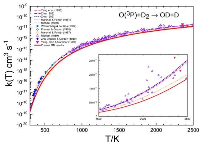
**Fig. 10** Comparison of individual measurements<sup>8,13,15,19,23,24</sup> and global fits<sup>15,16,19,23</sup> of rate coefficients for the O + D<sub>2</sub> reaction. The inset shows a blow-up of the 1500–2500 K range. The red solid line represents the present QM  $k(T)$ .
