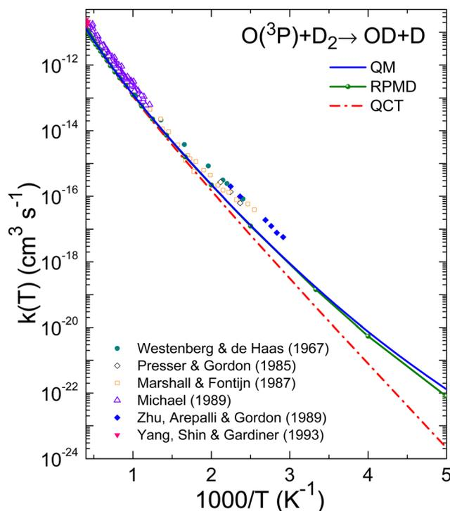
Fig. 8 Same as Fig. 7 for the  $\text{O}(^3\text{P}) + \text{D}_2$  reaction. Experimental results: Westenberg and de Haas,<sup>8</sup> Presser and Gordon,<sup>13</sup> Marshall and Fontijn,<sup>15</sup> Michael,<sup>23</sup> Zhu *et al.*<sup>24</sup> and Yang *et al.*<sup>19</sup>
