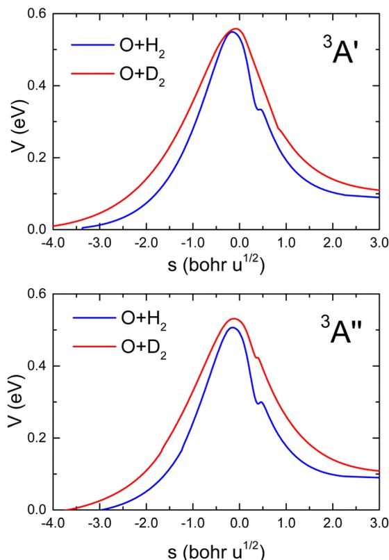
Fig. 1 Vibrational adiabatic minimum energy paths for  $\text{O}(^3\text{P}) + \text{H}_2$  (blue) and  $\text{O}(^3\text{P}) + \text{D}_2$  (red) reactions as a function of the mass-scaled reaction coordinate (see text for definition) on the  $^3\text{A}'$  (upper panel) and  $^3\text{A}''$  (bottom panel) PESs calculated by Zanchet *et al.*<sup>27</sup> In both cases, the minimum energy paths for the two isotopes are referred to as the respective ZPE of  $\text{H}_2$  and  $\text{D}_2$ .
