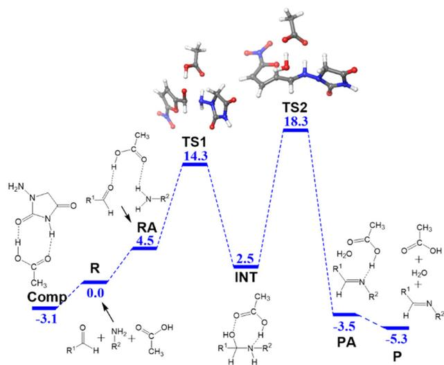
**Fig. 1** Free energy profile in kcal mol<sup>-1</sup> for the formation of nitrofurantoin in water. The highlighted species are: acetic acid:1-amino-hydantoin complex (**Comp**), reactants (**R**), reactant adduct (**RA**), transition states (**TS**), intermediate (**INT**), product adduct (**PA**), and products (**P**). The same abbreviations will be used in the figures below. The structures of **TS** are highlighted in 3D. Color scheme: O (red), N (blue), C (grey), and H (white).
