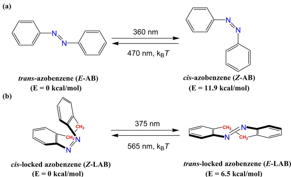
**Scheme 1** Schematic representation of *cis*(*Z*)/*trans*(*E*) photoisomerization of (a) azobenzene (AB)<sup>34</sup> and (b) locked azobenzene (LAB)<sup>13</sup> and their relative energies with respect to the most stable isomer calculated at SA2-CASPT2(14,12)/6-31G(d)//CASSCF(14,12)/6-31G(d) for AB<sup>35</sup> and at MS-SA2-CASPT2(6,4)/6-31G(d)//SA2-CASSCF(6,4)/6-31G(d) for LAB<sup>36</sup> are given.
