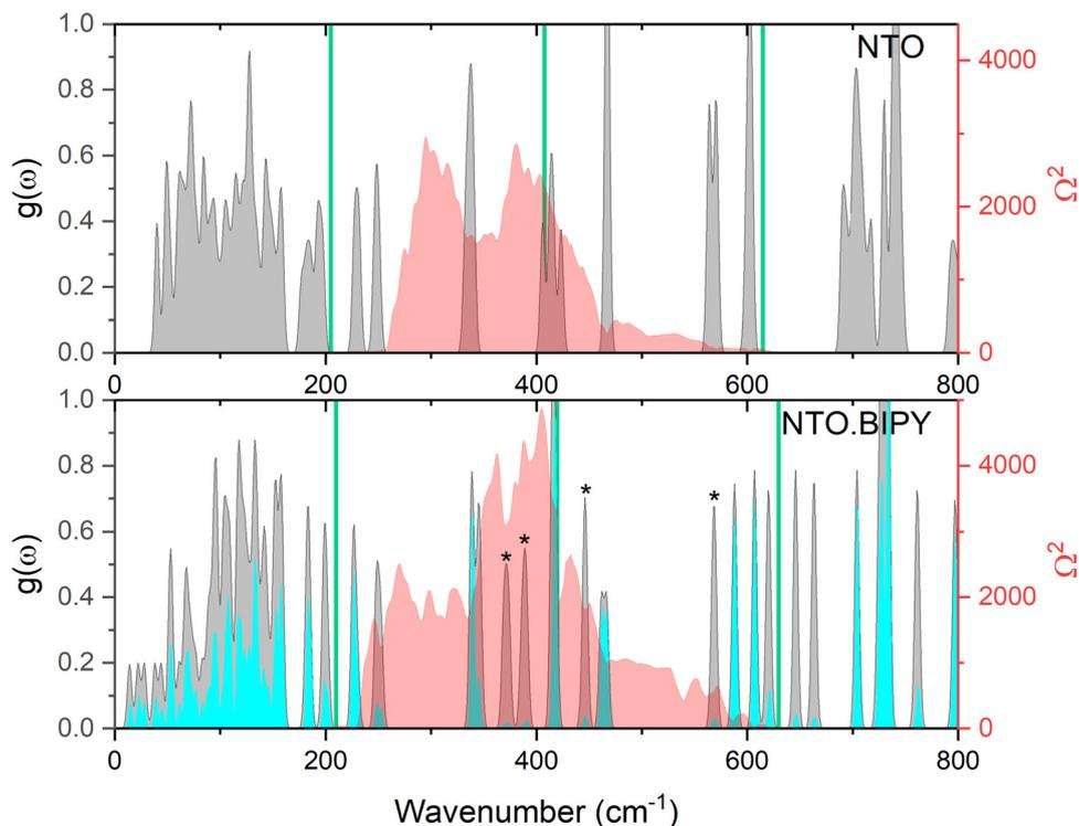
Fig. 9 Simulated  $g(\omega)$  (grey), and corresponding  $\Omega^{(2)}$  (red) for NTO (top)<sup>27</sup> and NTO-BIPY (bottom) at ambient conditions. The partial  $g(\omega)$  for NTO in the co-crystal is shown in cyan, and peaks with negligible NTO character are marked with an asterisk. The green vertical lines represent sequential multiples of  $\Omega_{\max}$ , within an  $1-3 \Omega_{\max}$  up-pumping window.
