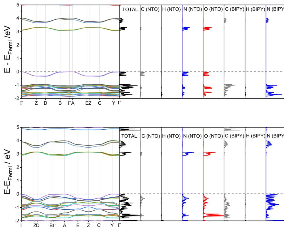
Fig. 5 Calculated electronic band structures for NTO-BIPY, alongside partial density of states (top: 0 GPa, bottom 5.93 GPa). The dotted black line indicates the Fermi level, set to 0 eV in each case (absolute  $E_{\text{Fermi}}$  values: 0 GPa =  $-6.02$  eV; 5.93 GPa =  $-5.61$  eV).
