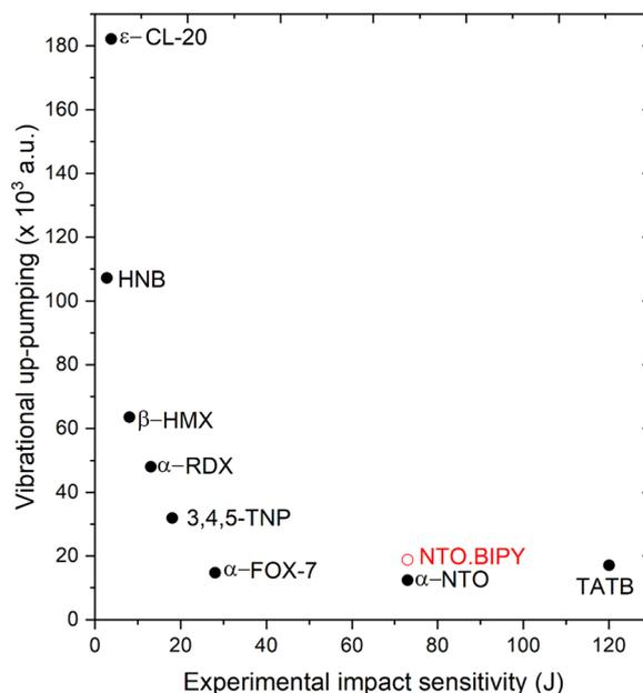
Fig. 10 Vibrational up-pumping densities vs. experimental IS values for a range of previously reported EMS<sup>26,27,39</sup> alongside the prediction for NTO-BIPY (shown in red). Filled symbols correspond to experimentally determined data, unfilled to predicted values only.
