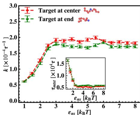
Fig. 8 The target search rate,  $k$ , is plotted as a function of non-specific interaction strength,  $\epsilon_{ns}$ , when the central bead is spatially fixed on a flexible DNA with the target at the center (red ‘-●-’ line), and at one of the ends (green ‘-▲-’ line).
