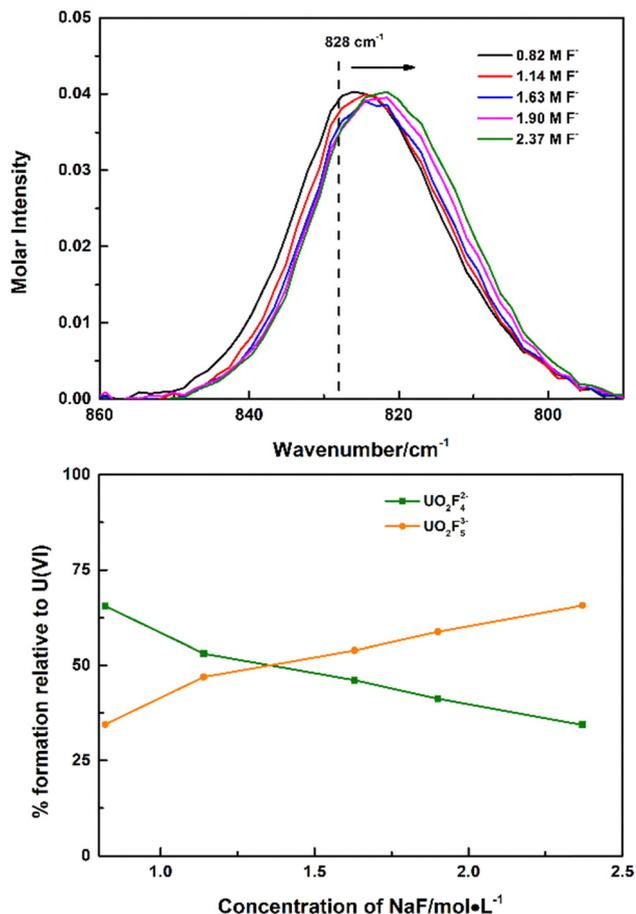
Fig. 2 Raman spectra of  $\text{UO}_2(\text{NO}_3)_2$  in 2.5 M  $(\text{CH}_3)_4\text{NNO}_3/(\text{CH}_3)_4\text{NNO}_3$  (top) and speciation distribution during titration (bottom).  $C_{\text{Uranyl}} = 0.059$  M,  $C_{\text{Nitrate}} = 0.118\text{--}1.69$  M,  $V = 1.0$  mL,  $C_{\text{H}^+} = 0.002$  M,  $C_{\text{Fluoride}} = 0.82\text{--}2.37$  M.
