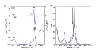
Fig. 8 (a) MCD (top) and electronic absorption (bottom) spectra of Co windmill complex in CHCl<sub>3</sub> at room temperature. (b) Electronic absorption spectra during the electrochemical reduction of windmill at -0.8 V (vs. Ag/ AgCl) in benzonitrile with 0.1 M n-Bu<sub>4</sub>NPF<sub>6</sub> under a nitrogen atmosphere.
