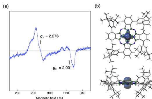
Fig. 11 (a) ESR spectrum of Co windmill in benzonitrile at 77 K under Ar. The sample concentration was 0.5 mM. (b) Spin density map (isoval = 0.0004, blue: positive spin, green: negative spin) of the low-spin doublet state of Co windmill calculated at the UB3LYP/6-31G(d,p) level.
