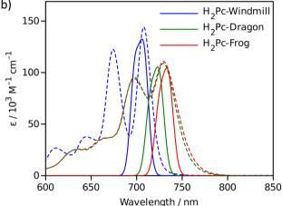
Fig. 6 Absorption spectra: (a) measured in toluene for free bases (solid lines) and cobalt complexes (dotted lines); (b) free base spectra (dotted lines) overlapped with the calculated absorption bands (solid lines)
