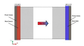
Fig. 3 The simulation model for the NEMD calculations of the thermal
