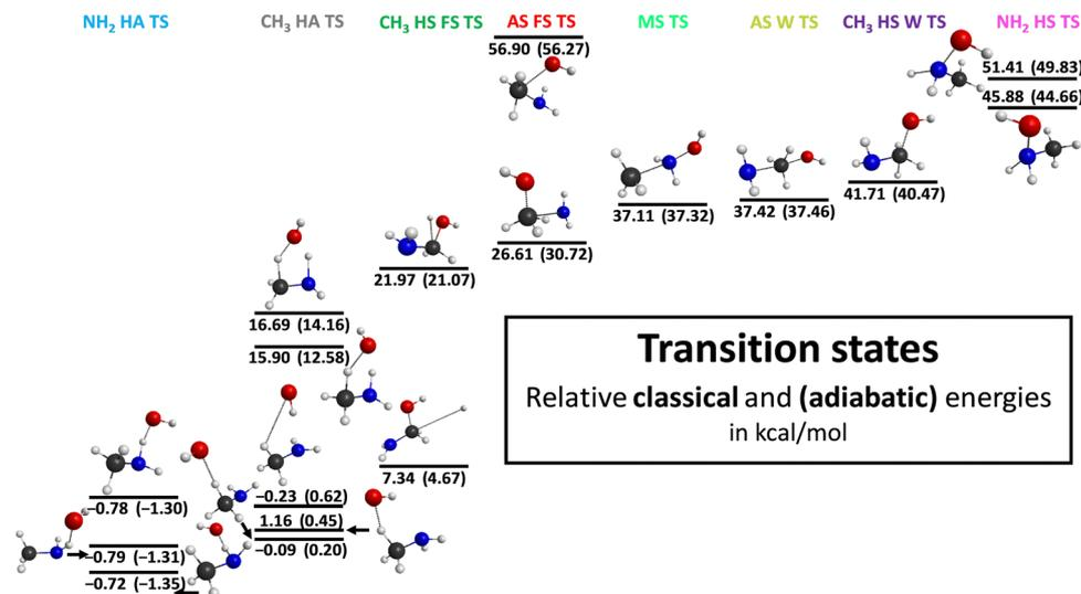
Fig. 3 Different transition state structures for the OH + CH<sub>3</sub>NH<sub>2</sub> reaction illustrating the benchmark classical and adiabatic energies relative to the reactants.
