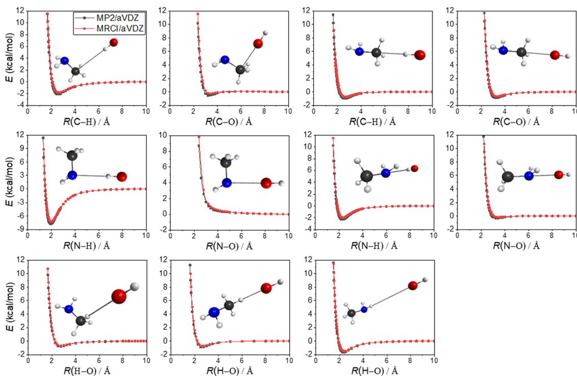
Fig. 1 Potential energy curves determined in different directions for the entrance channel at the levels of MP2/aug-cc-pVDZ (black) and MRCI/aug-cc-pVDZ (red) theory where the OH and  $CH_3NH_2$  molecules are kept frozen at their equilibrium structures and only one distance (dotted bond) is varied.
