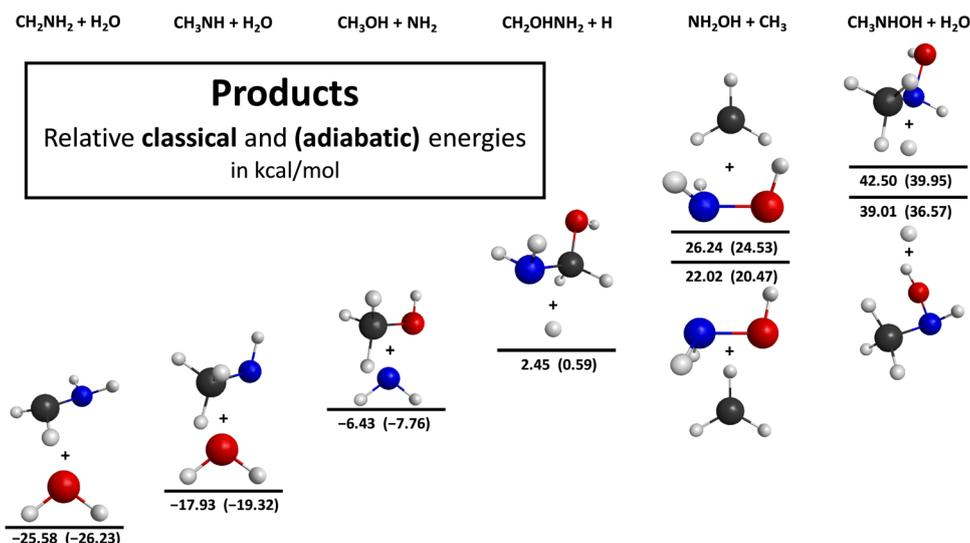
Fig. 5 Different product structures for the OH + CH<sub>3</sub>NH<sub>2</sub> reaction illustrating the benchmark classical and adiabatic energies relative to the reactants.
