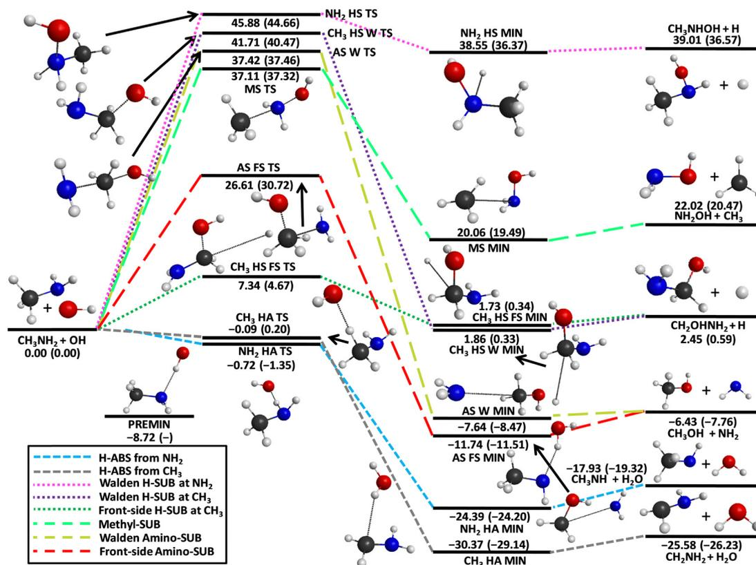
Fig. 2 Schematic potential energy surface of the  $\text{OH} + \text{CH}_3\text{NH}_2$  reaction visualizing the most accurate optimized geometries and classical (adiabatic) benchmark energies, in  $\text{kcal mol}^{-1}$ , of the lowest-energy conformers relative to the reactants.
