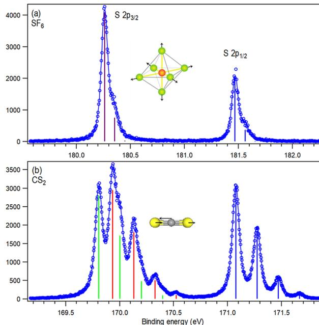
Fig. 5 Sulfur 2p near-threshold photoelectron spectra from  $\text{SF}_6$  (a) and  $\text{CS}_2$  (b). Vertical bars mark the positions and heights of fitted peaks, with colours differentiating the s–o and MF split components. Blue:  $2p_{1/2,1/2}$ , red:  $2p_{3/2,1/2}$  and green  $2p_{3/2,3/2}$ . Spectrum (b) and its fitting results are reproduced from ref. 13. The inset graphics illustrate the Franck–Condon-excited vibrational modes.
