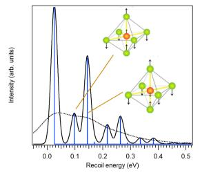
Fig. 2 Simulated recoil lineshape for the S 2p photoemission from SF6 for  $h\nu$  = 7 keV at the temperature of 30 K and with no lifetime broadening (solid line) and at 300 K including the lifetime broadening (dotted line). The latter will be assigned to each Franck-Condon transition in describing experimental HAXPES spectra.
