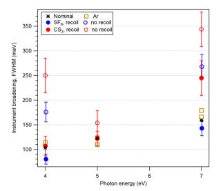
Fig. 8 Instrumental broadenings (full-width at half-maximum) in the HAXPES spectra, as determined by least-squares fitting and compared to the nominal values of the instrumental resolution. Multiple values for Ar 2p result from different series of measurements. The error bars reflect only the statistical error in the least-squares fitting
