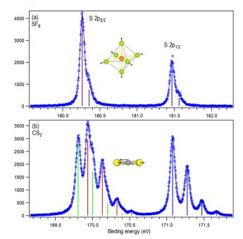
Fig. 5 Sulfur 2p near-threshold photoelectron spectra from SF6 (a) and CS<sub>2</sub> (b). Vertical bars mark the positions and heights of fitted peaks, with coulours differentiating the s-o and MF split components. Blue: 2p<sub>1/2,1/2</sub>, red:  $2p_{3/2,1/2}$  and green  $2p_{3/2,3/2}$ . Spectrum (b) and its fitting results are reproduced from ref. 13. The inset graphics illustrate the Franck-Condonexcited vibrational modes.
