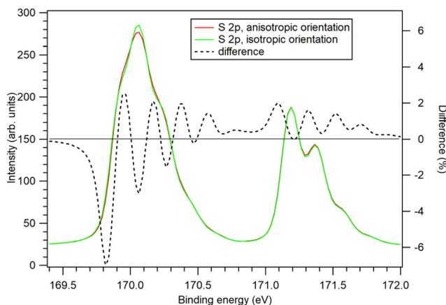
Fig. 9 Generated S 2p photoelectron spectra for  $h\nu = 7$  keV, using the fitted structure of Fig. 8(b), but reducing the temperature to 70 K and instrumental broadening to 60 meV (equal to the lifetime broadening). Red: using the theoretically predicted molecular orientation distributions for and green: using isotropic distributions for all components. The black dashed line is the difference between the first and the second spectrum.
