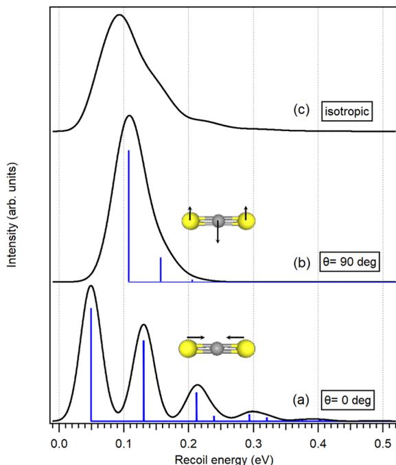
**Fig. 3** Simulated recoil lineshapes for the S 2p photoemission from CS<sub>2</sub> for  $h\nu = 7$  keV, at  $T = 30$  K and without lifetime broadening. Shape (a) corresponds to axial emission direction, (b) to perpendicular emission in respect to the molecular axis and (c) to isotropic emission. The latter would be assigned to each Franck–Condon transition in describing the experimental HAXPES spectrum, if the anisotropy effects can be neglected.
