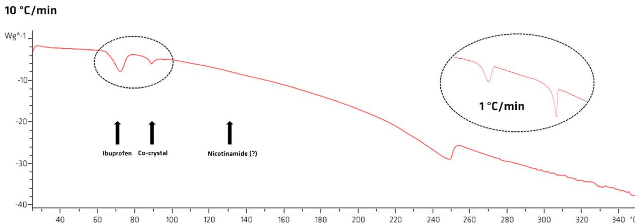
Fig. 6 10 °C min<sup>-1</sup> DSC trace for the physical mixture ibuprofen–nicotinamide. It is evidenced the melting point of ibuprofen (78 °C), of the co-crystal (90 °C) and the one – missing – of nicotinamide (130 °C). In the black dashed circle on the right, the 1 °C min<sup>-1</sup> DSC of the physical mixture to better appreciate the formation of the co-crystal among melting.
