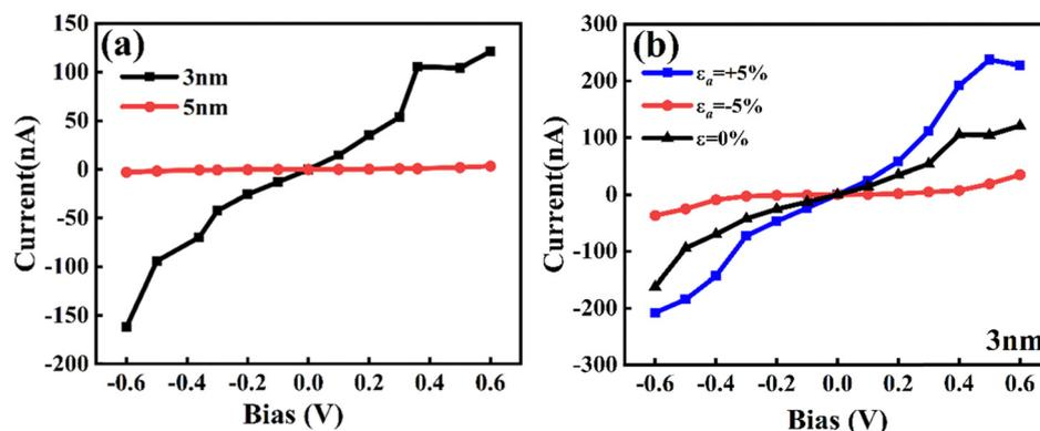
Fig. 6 The  $I$ - $V$  characteristic curves of  $\text{Si}_9\text{C}_{15}$ , including (a) those along the  $a$  direction for  $L_c$  of 3 nm and 5 nm without applied strain, and (b) those for a  $L_c$  of 3 nm along the  $a$  direction with applied strains of 5% and  $-5\%$ .
