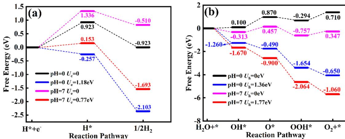
Fig. 10 Free energy diagrams for the (a) two-electron pathways of the HER and (b) four-electron pathways of the OER in the  $\text{Si}_9\text{C}_{15}$  at pH = 0 and 7 and different external potential energy.
