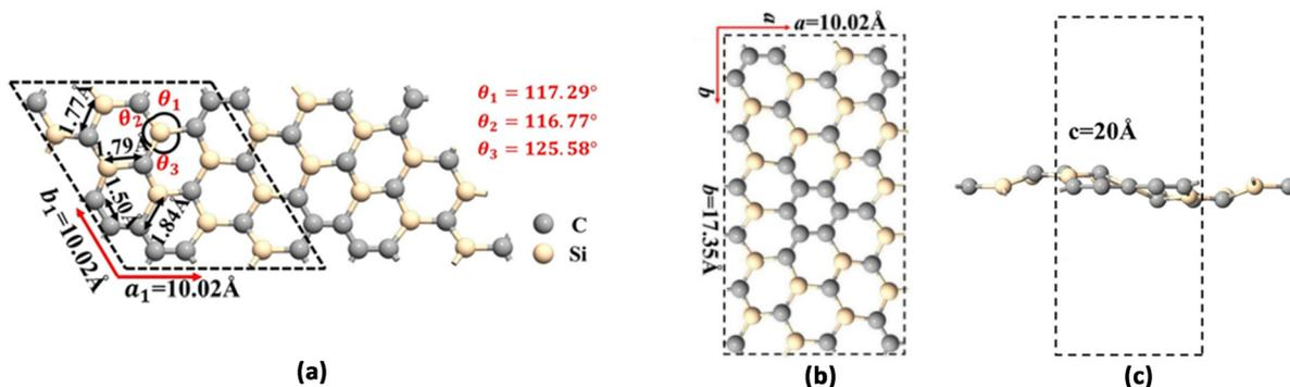
Fig. 1 (a) Top view of the hexagonal unit cell, (b) side view of the hexagonal unit cell, (c) orthogonal supercell of Si<sub>9</sub>C<sub>15</sub>.
