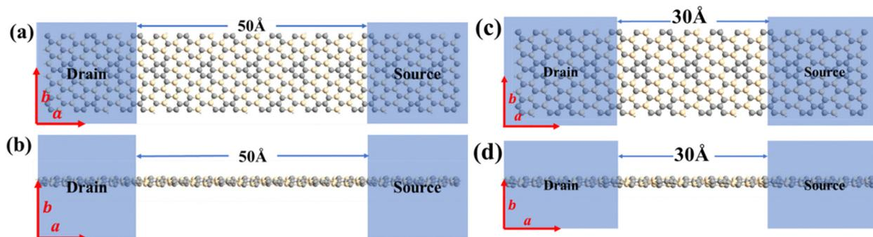
Fig. 5 The schematic diagram of two-electrode system with  $L_c$  of 5 nm and 3 nm, including (a) the top and (b) the side views of the 5 nm configuration, (c) the top and (d) the side views of the 3 nm configuration.
