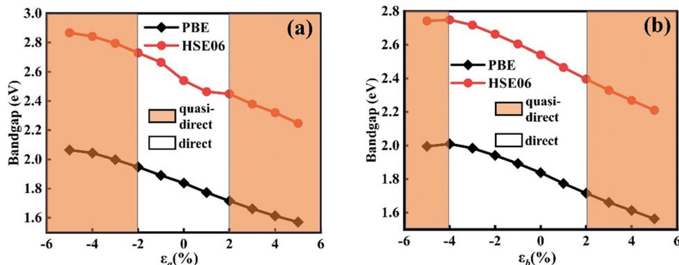
Fig. 3 The bandgap variation of  $\text{Si}_9\text{C}_{15}$  after applying  $-5\%$  to  $5\%$  strain along the (a)  $a$  direction and (b)  $b$  direction, where the white and orange regions represent the strain ranges corresponding to direct and quasi-direct bandgaps, respectively.
