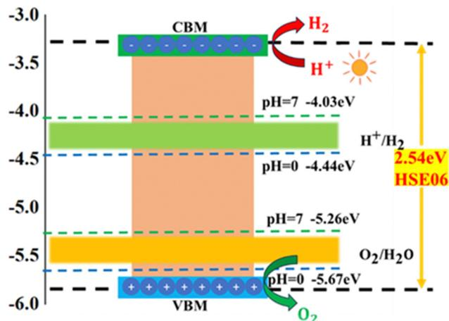
Fig. 9 The band edge positions relative to the vacuum energy level of  $\text{Si}_9\text{C}_{15}$  using HSE06. The green and blue dashed lines represent the reduction potential and oxidation potential at pH = 7, 0, respectively.
