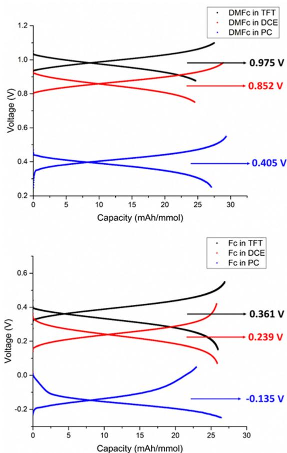
**Fig. 2** Charge and discharge profiles from battery experiments. top) Comparing decamethylferrocene (DMFc) in trifluorotoluene (TFT), dichloroethane (DCE), and propylene carbonate (PC). bottom) Comparing ferrocene (Fc) in the same solvents.
