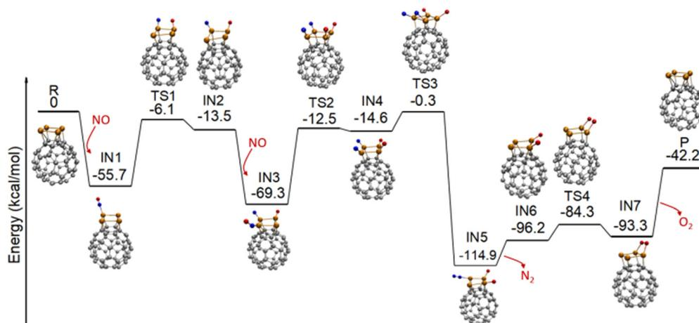
Fig. 1 Reaction pathway of NO reduction on  $\text{C}_{60}\text{Rh}_4^+$  calculated at the BPW91/6-31G(d)&SDD level of theory. R stands for reactants, IN for intermediates, TS for transition states, and P for products. All energies are provided relative to the energies of the reactants, *i.e.*,  $\text{C}_{60}\text{Rh}_4^+$  and two NO molecules.
