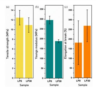
Fig. 8 Variation of the mechanical properties: (a) Tensile strength. (b) Youngs modulus. (c) Elongation at break of the LPO and LP30 samples.
