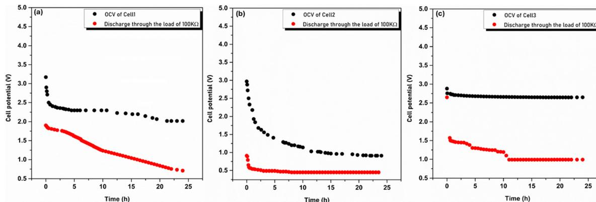
Fig. 9 Open circuit voltage and discharge characteristics of Cell 1 (a), Cell 2 (b) and Cell 3 (c).
