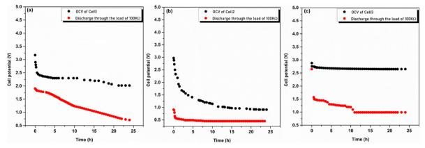
Open circuit voltage and discharge characteristics of Cell 1 (a), Cell 2 (b) and Cell 3 (c).
