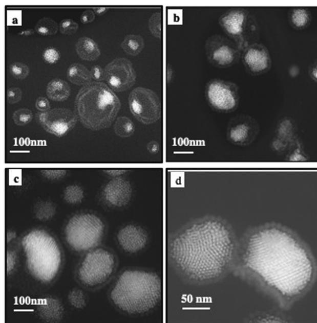
Fig. 5 2D HAADF-STEM (a)–(d) overview of superstructures of 10 nm  $\text{Fe}_3\text{O}_4$  nanocrystals ( $2 \text{ mg mL}^{-1}$ ) and 5 nm Au nanocrystals differing by their amounts: (a)  $10 \text{ mg mL}^{-1}$ , (b)  $60 \text{ mg mL}^{-1}$ , (c)  $100 \text{ mg mL}^{-1}$  and (d)  $200 \text{ mg mL}^{-1}$ .
