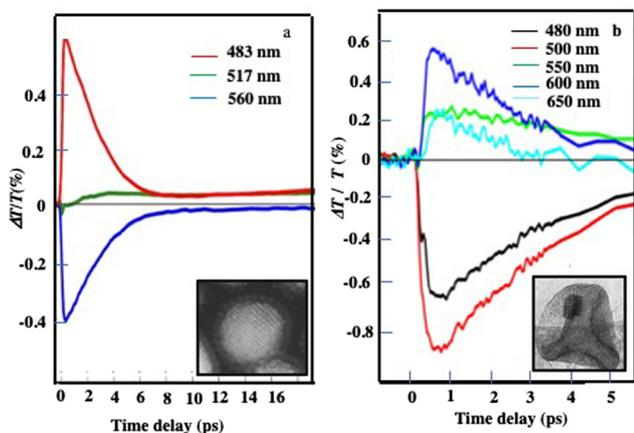
Fig. 12 Dynamics of the  $\Delta T/T$  at selected probe wavelengths, at short time scales of energy flow in the (a) Au and (b)  $\text{Au}(\text{Fe}_3\text{O}_4)_{13}$  superstructures.<sup>27</sup>
