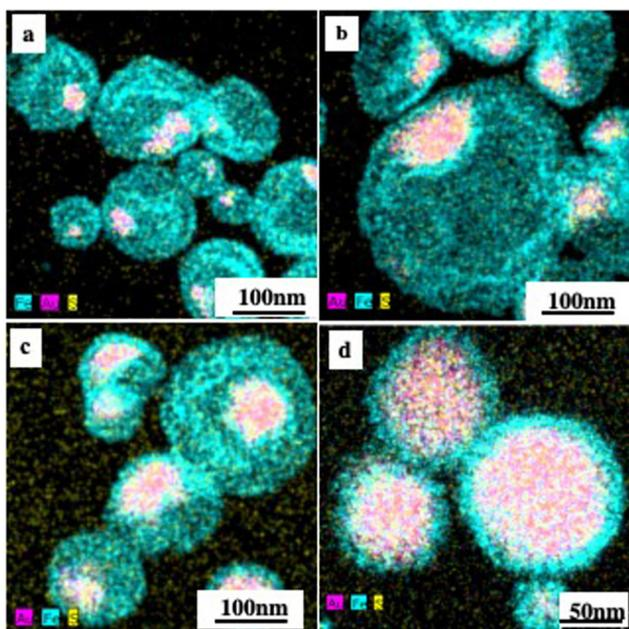
Fig. 7 EDS mapping (a)–(d) overview of "egg" superstructures of 10 nm Fe<sub>3</sub>O<sub>4</sub> nanocrystals (2 mg mL<sup>-1</sup>) and 5 nm Au NCs differing by their amounts such as 10 mg mL<sup>-1</sup> (a), 60 mg mL<sup>-1</sup> (b), 100 mg mL<sup>-1</sup> (c) and 200 mg mL<sup>-1</sup> (d). Cyan, magenta and yellow denote Fe, Au and S elements respectively.
