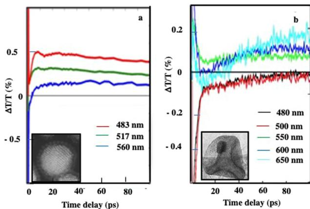
Fig. 13 Dynamics of the  $\Delta T/T$  at selected probe wavelengths, at long-time scales of energy flow in the (a) Au and (b)  $\text{Au}(\text{Fe}_3\text{O}_4)_{13}$  superstructures.<sup>27</sup>
