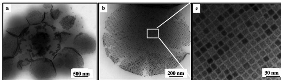
Fig. 3 TEM images of a colloidosome of  $\text{Fe}_3\text{O}_4$  nanocubes at different scales.<sup>20</sup>
