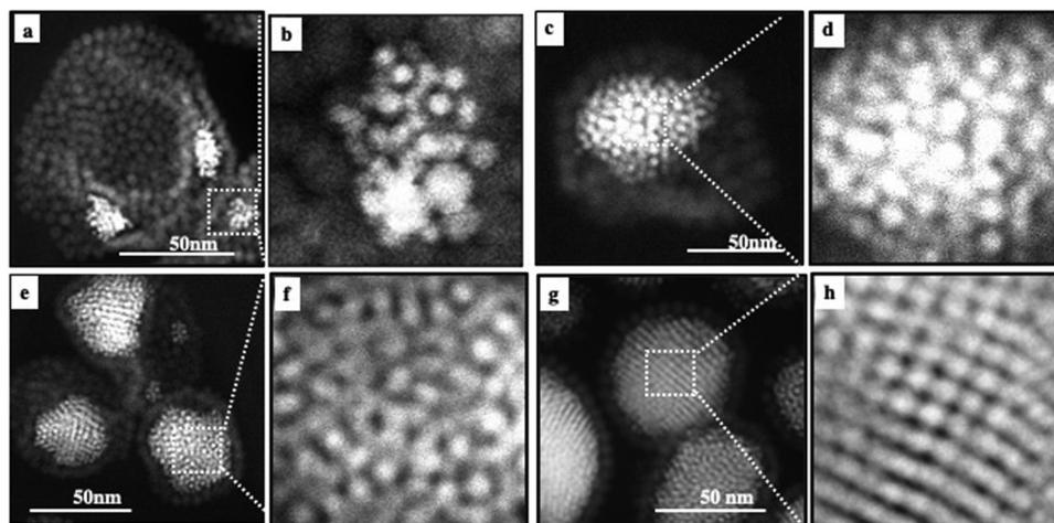
Fig. 6 High resolution 2D HAADF-STEM images (a), (c), (e) and (g) and enhancement of the nanocrystal ordering (b), (d), (f) and (h) of 10 nm Fe<sub>3</sub>O<sub>4</sub> nanocrystals (2 mg mL<sup>-1</sup>) and 5 nm Au nanocrystals differing by their amounts: (a) and (b) 10 mg mL<sup>-1</sup>, (c) and (d) 60 mg mL<sup>-1</sup>, (e) and (f) 100 mg mL<sup>-1</sup> and (g) and (h) 200 mg mL<sup>-1</sup>.
