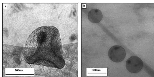
Fig. 8 Cryo-TEM image of a single colloidosome assembled from the Fe<sub>3</sub>O<sub>4</sub>/Au binary mixture.<sup>20</sup>
