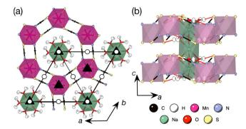
Fig. 1 Neutron single crystal structure of [Na(OH<sub>2</sub>)<sub>3</sub>]Mn(NCS)<sub>3</sub> (D19 at the ILL, 25 K). <sup>17</sup> (a) View along the c axis. Space group diagram for  $P\overline{3}$  overlaid,  $\bar{1}$ : white circle, 3: black triangle. (b) View along the b axis. Hydrogen bonds shown as red lines
