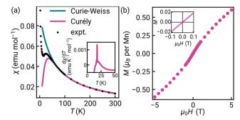
Fig. 2 (a) Magnetic susceptibility,  $\chi$  measured from 2–300 K (black), with the high temperature fits using the Curie-Weiss (teal) and Curély equation (pink) for a classical honeycomb magnet. Inset: Temperature derivative of the susceptibility in the vicinity of the transition. (b) Isothermal magnetisation data, measured between +5.00 and -5.00 T at 2 K. Inset: Close-up of data between +0.1 and -0.1 T.
