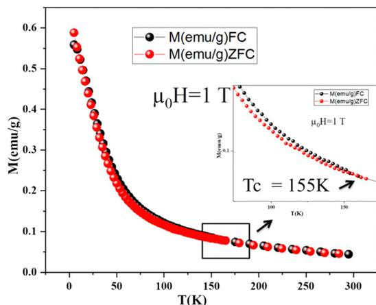
Fig. 11 Temperature dependence of the  $M(\text{FC})$  and  $(\text{ZFC})$  magnetization of LSSiRuO compound under  $\mu_0H = 1 \text{ T}$ . (The inset shows the local enlargement where ZFC and FC curves begin to diverge.)
