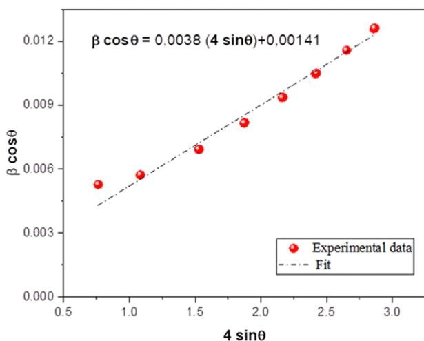
**Fig. 2** Williamson–Hall (W–H) plot of  $\text{La}_{0.25}\text{Sr}_{0.75}\text{Sn}_{0.4}\text{In}_{0.25}\text{Ru}_{0.35}\text{O}_3$ .
