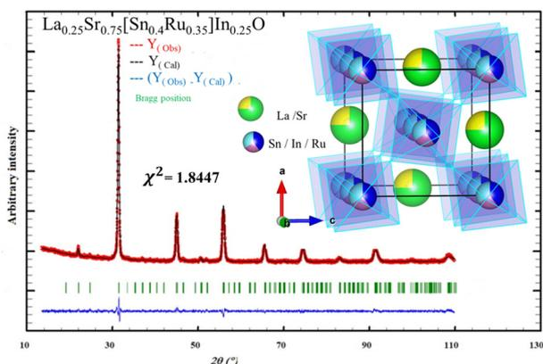
**Fig. 1** Observed, calculated and difference of X-ray diffraction patterns of  $\text{La}_{0.25}\text{Sr}_{0.75}\text{Sn}_{0.4}\text{In}_{0.25}\text{Ru}_{0.35}\text{O}_3$  powder calcined at 1050 °C with structure inset.
