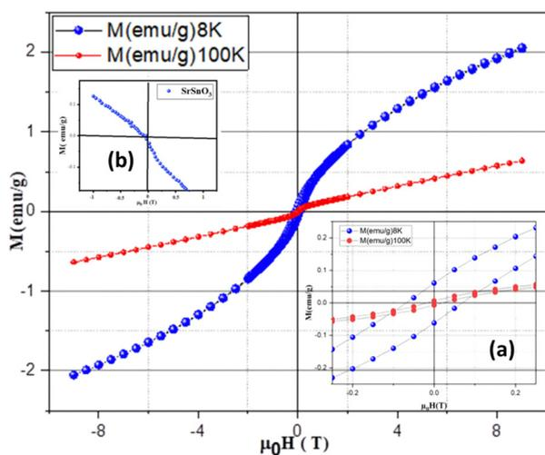
Fig. 12 Magnetization dependence of LSSiRuO as a function of the magnetic field. (Inset: (a) an enlarged view of the central region of the curves; (b) magnetisation of  $\text{SrSnO}_3$ .<sup>60</sup>)
