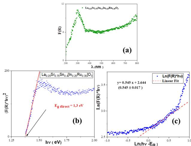
Fig. 6 (a) Kubelka–Munk function  $F(R)$  for  $\text{La}_{0.25}\text{Sr}_{0.75}\text{Sn}_{0.4}\text{In}_{0.25}\text{Ru}_{0.35}\text{O}_3$  as a function of wavelength  $\lambda$ . (b) Tauc plot for  $\text{La}_{0.25}\text{Sr}_{0.75}\text{Sn}_{0.4}\text{In}_{0.25}\text{Ru}_{0.35}\text{O}_3$ . (c) Plot of  $\ln(F(R) \times hv)$  vs.  $\ln(h\nu - E_g)$ .
