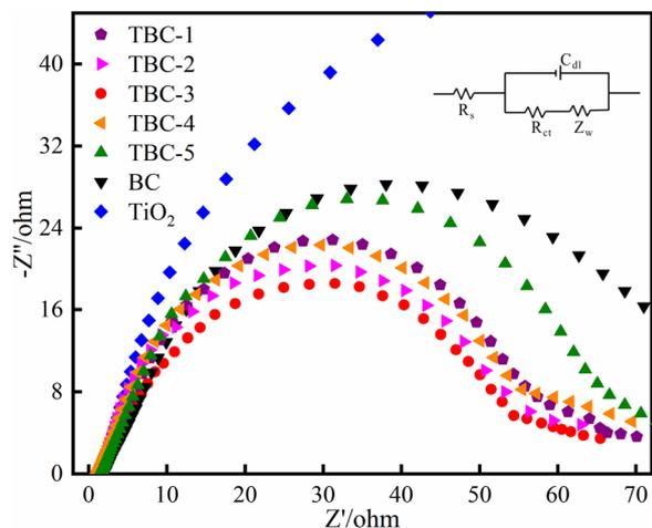
Fig. 7 EIS Nyquist plots of the as-prepared BC, TiO<sub>2</sub>, and TBC samples in 1 M Na<sub>2</sub>SO<sub>4</sub> solution and the inset shows the equivalent circuit fitting of EIS data.
