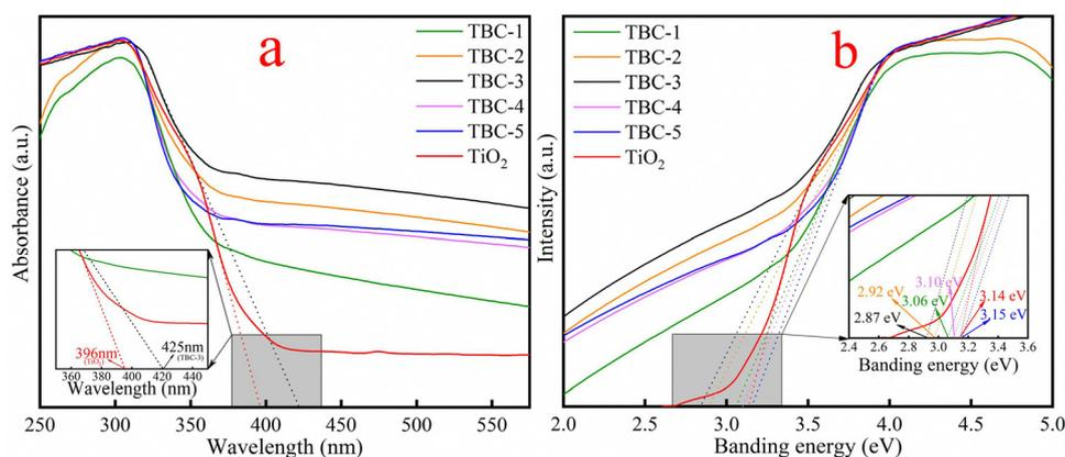
Fig. 3 UV-Vis absorption spectra (a) and corresponding band gap energies (b) of TiO<sub>2</sub> and TBC samples.
