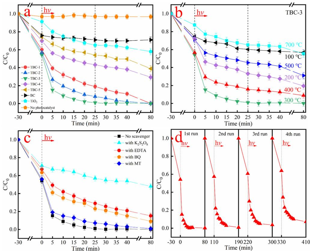
Fig. 9 Adsorption-photocatalytic reduction of Cr(vi) with BC, TiO<sub>2</sub> and TBC samples (a), with TBC-3 calcined at different temperatures (b) and over TBC-3 composite in the presence of K<sub>2</sub>S<sub>2</sub>O<sub>8</sub>, EDTA, BQ and MT scavengers (c). Recycling experiments using TBC-3 composite for the adsorption-photocatalytic reduction of Cr(vi) (d).
