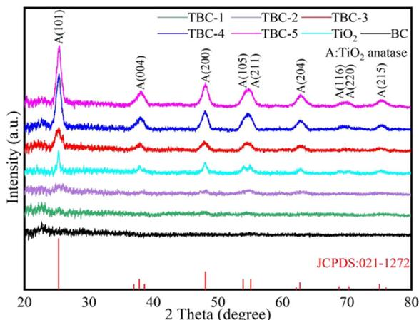
Fig. 1 XRD patterns of BC, TiO<sub>2</sub> and TBC samples.
