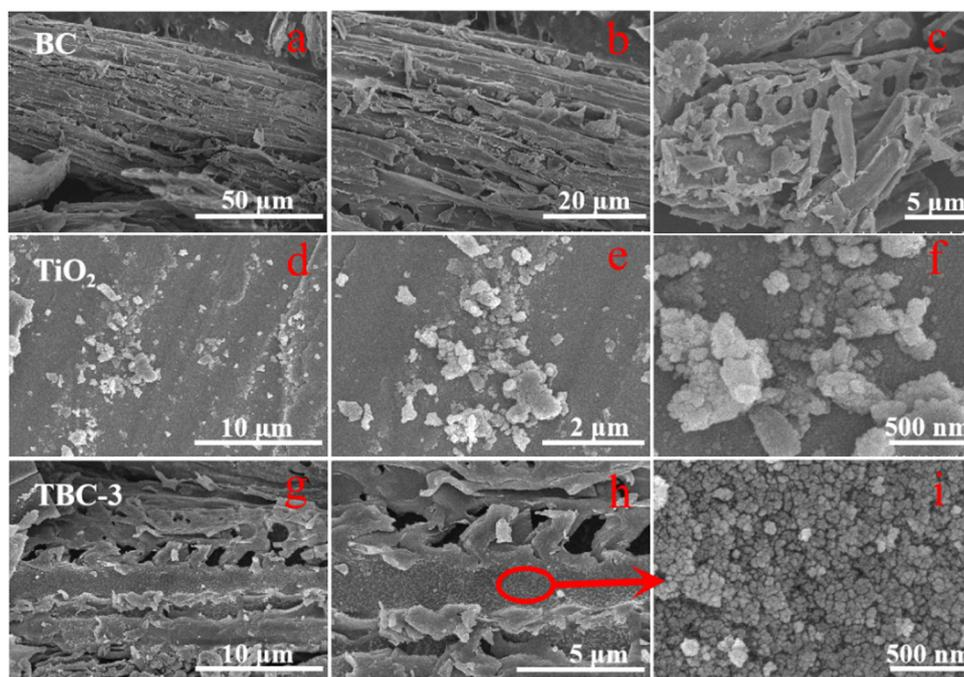
Fig. 4 Typical SEM images of the as-prepared samples. SEM images of BC (a)–(c), TiO<sub>2</sub> (d)–(f) and TBC-3 (g)–(i).
